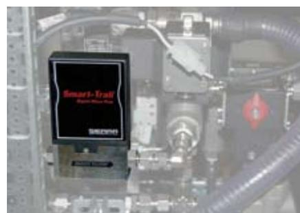
Figure 4: A Smart-Trak mass-flow meter and controller
