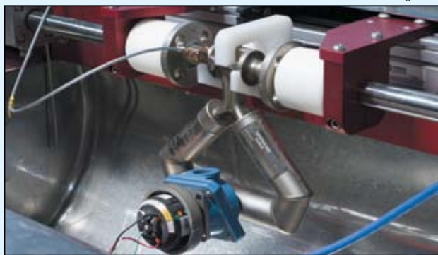
A Micro Motion Elite flowmeter gets calibrated at Emerson's European Flow Center at Ede, Netherlands
