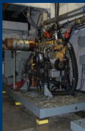
John Deere Test Engine Equipped with Johnson Matthey CCRT ® Installed on Engine Dynamometer Testing Platform
