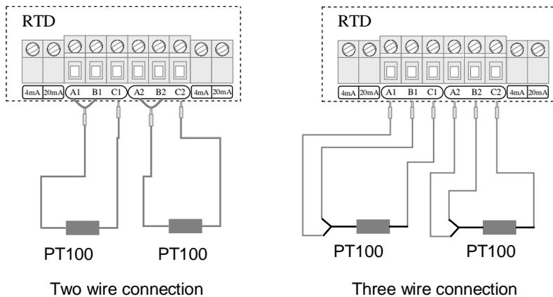
The two PT100 temperature sensors are installed on the inlet and return pipes and they will input temperature signals to the SIERRA 205 transmitter.
