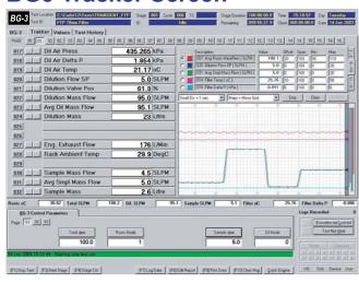
The "Tracker" function is a tool that every engineer will find irreplaceable. This screen can be used by the engineer to track any of the functions (diluted mass flow, delta pressure, engine exhaust flow versus sample mass flow) or other immediate test functions for immediate reference or archival of data.
