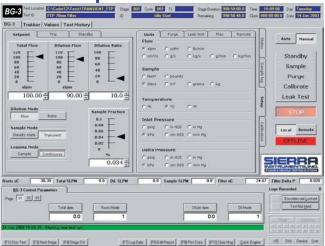
The BG3 set-up screen is unique in that it can be modified for any test situation. Altering the units of measure is one of the easily adjustable features of the set-up screen. The easily accessed (tab) screen allows the engineer the rapid change of any test parameter.
