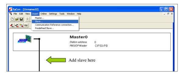
2. Set the slave filter to "Sierra Instruments Inc." Select the desired GSD file, press the "Add" button, set the slave address and description to match the slave and press the "OK" button.
