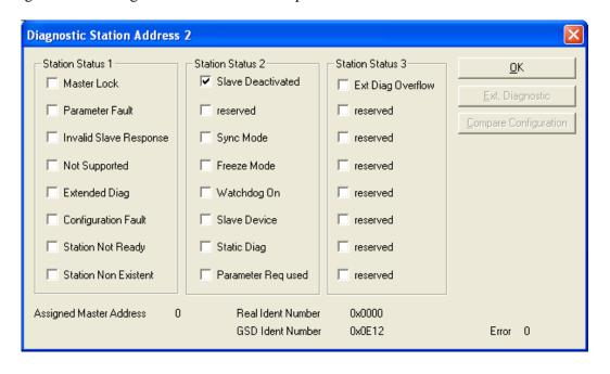
In this case the slave is deactivated. Check the address of "Slave1" to see if it matches with the physical address of the hardware slave.
