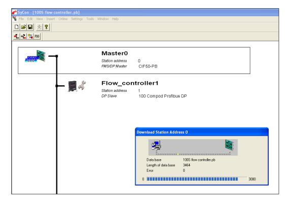
When done save the new configuration to disk (File -> save as). Put the .pb file where your server can get it later. The system is ready to be used.
