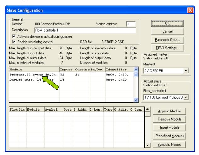
4. Select the desired modules by double clicking on the module name. Press the "OK" button.
