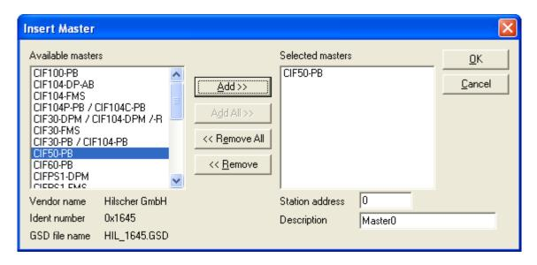
Leave the station address set to zero. Press the "Add" button and then the "OK" button.
