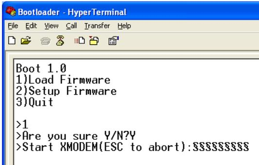
3. The screen will start to fill up with the “\$” character indicating that the XMODEM transfer can be started. Press the “ESC” key to abort (if needed).
