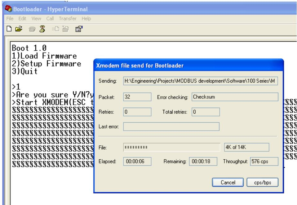
10. When the download is finished, the start-up menu screen will be appear again presenting three the original three options: 1) Load Firmware, 2) Setup Firmware, and 3) Quit.
