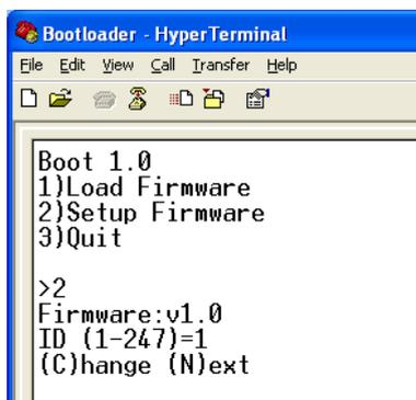
Also, shown on this screen is the version of the firmware, the first option which you can set, the currently selected value ID values, and what values you can select to change. In this above example, the ID code of the unit can be set between 1- 247. The current setting for the ID is 1.
