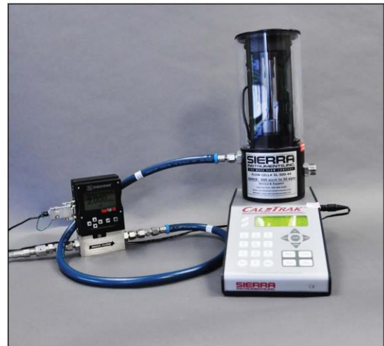
CalTrak MFM/MFC Calibration Setup
