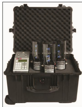
CalTrak Base with Three Flow Cells
