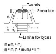
Figure 1-1. Flow Paths through the Instrument
