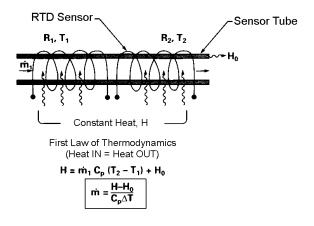
Figure 1-2. Flow Measuring Principle
