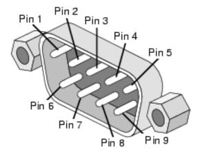
DB9 Pin-out locations on instrument. There are two DB9 connectors, one on each side of the enclosure.
