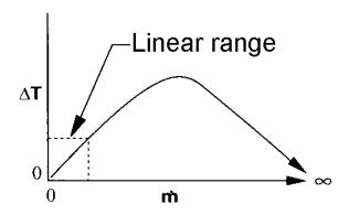
Figure 1-4. Linear Range of the Transducer's Output Signal
