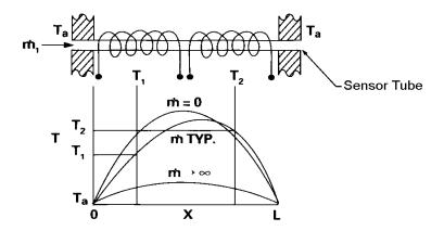
Figure 1-3. Sensor Temperature Distribution
