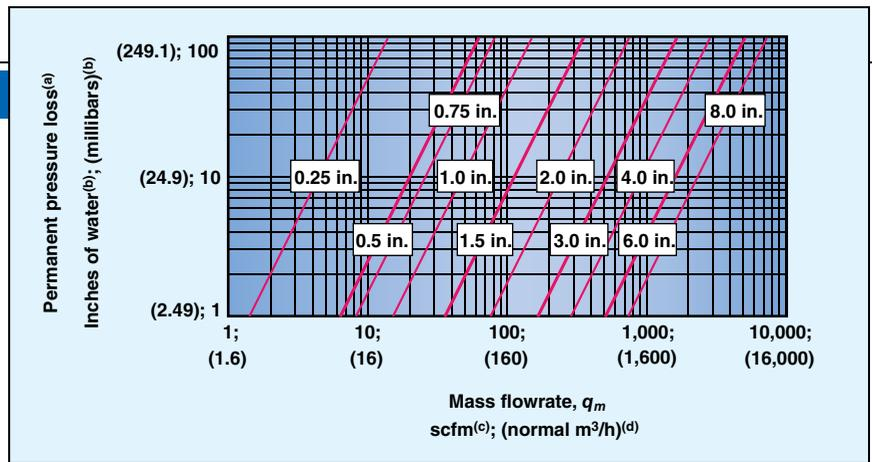
**FIGURE 6.** This graph shows the permanent pressure loss for in-line flowmeters with a built-in flow conditioner consisting of two upstream separated perforated plates. Notes: (a) for air and nitrogen at 21.1°C and 1 atm; (b) 1 in. of water = 0.0361 psi; (c) at standard conditions of 21.1°C and 1 atm; and (d) at standard (normal) conditions of 0°C and 1 atm
