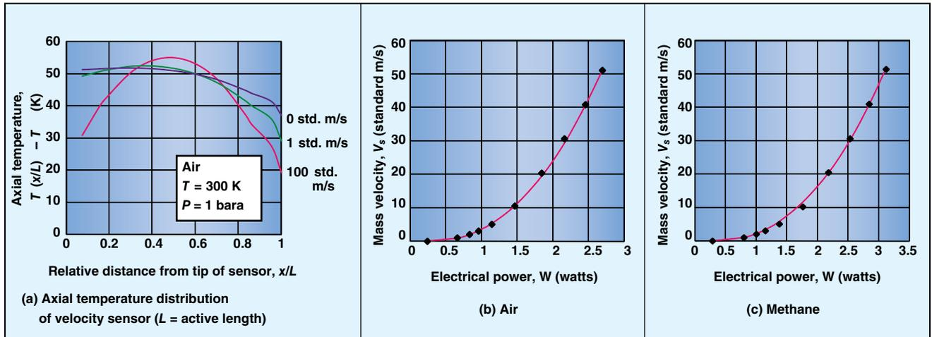
**FIGURE 5.** These plots compare flow calibration data and the output of the four-temperature microprocessor-based system.  $\Delta T = 50\text{K}$ , and  $T$  and  $P$  are at room (ambient) conditions. “Standard” conditions for  $V_s$  (standard m/s) are  $70^\circ\text{F}$  and 1 atm
