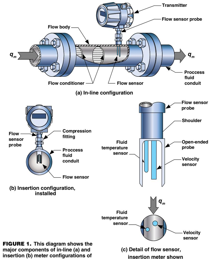
**FIGURE 1.** This diagram shows the major components of in-line (a) and insertion (b) meter configurations of thermal dispersion mass flowmeters
