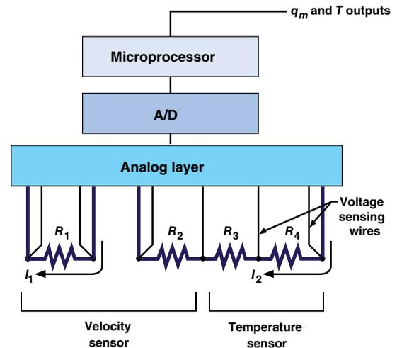
**FIGURE 3.** In the four-temperature microprocessor-based system, the flowmeter drives the velocity sensor so that the temperature difference  $\Delta T = T_1 - T$  is maintained constant. The system automatically corrects for changes in gas selection, gas temperature and gas pressure
