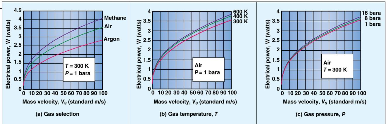
**FIGURE 4.** These plots show the management of changes in gas selection, gas temperature, and gas pressure with the four-temperature microprocessor-based system.  $\Delta T = 50\text{K}$ . In all figures the “standard” conditions for  $V_s$  (standard m/s) are  $70^\circ\text{F}$  and 1 atm
