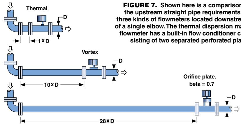
**FIGURE 7.** Shown here is a comparison of the upstream straight pipe requirements for three kinds of flowmeters located downstream of a single elbow. The thermal dispersion mass flowmeter has a built-in flow conditioner consisting of two separated perforated plates
