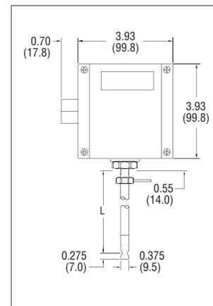
All dimensions are inches. Millimeters are in parentheses. Certified drawings are available on request.
