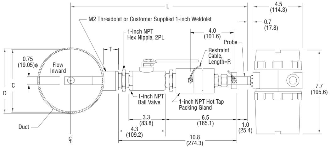
All dimensions are inches. Millimeters are in parentheses. All drawings have a +/-0.25-inch (6.4 mm) tolerance. Certified drawings are available on request.
