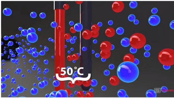
**Figure 1.** Thermal dispersion mass flow.
