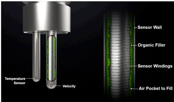
**Figure 3.** Wet sensor design.
