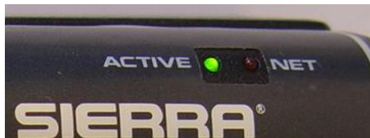
Figure 3 LED's showing the activities of the SmartTrak 100 Modbus™
