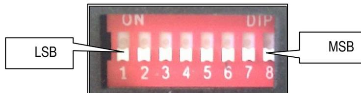
The switch becomes active when the slider is moved upwards. Here some examples of some addresses (1 = on/up, 0 = off/down):
