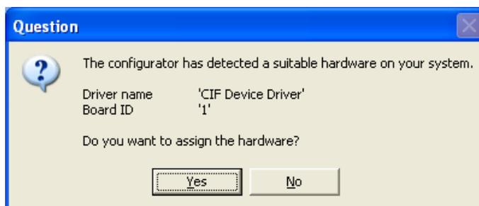
Note: The board ID number changes when extra PCI cards are added to the PC. Older configurations must be checked before trying to run them.
