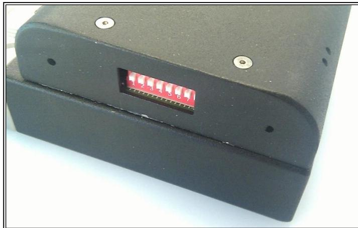
The dip switch is binary encoded with the LSB (lowest bit) on the left side. The switch is only read during power-up.
