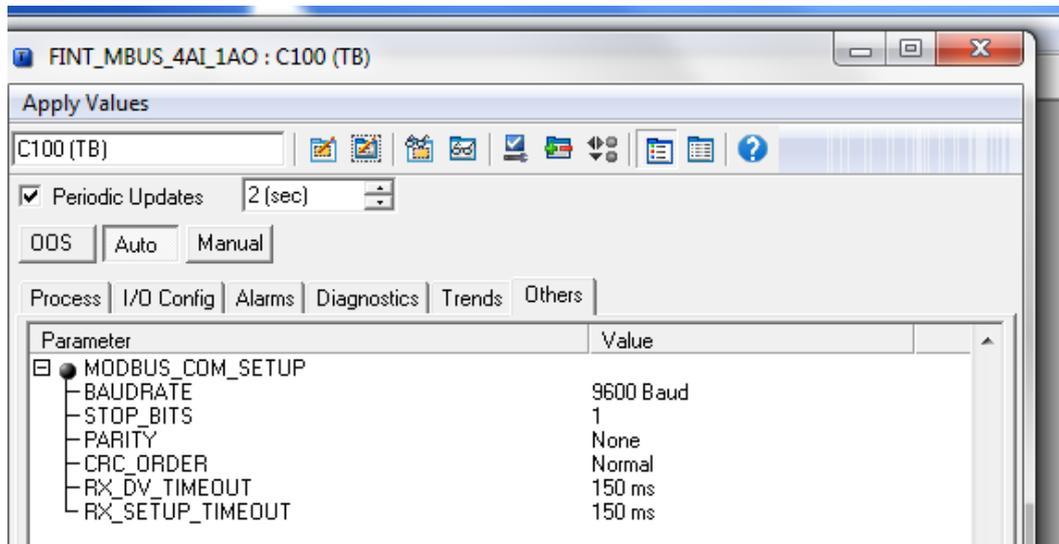
Figure 8: Screen Showing MODBUS\_COM\_SETUP
