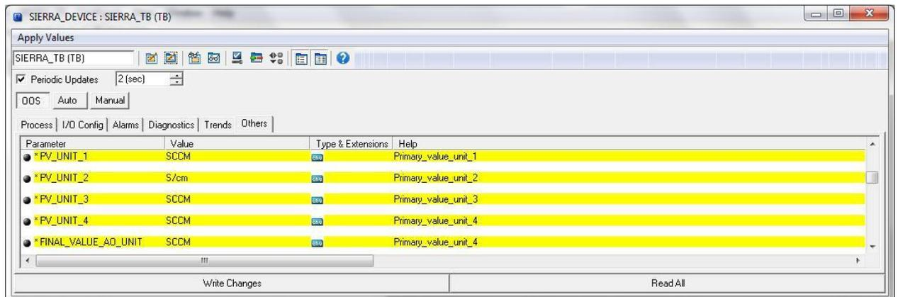
Figure 7: TB Block Engineering Units Setup
