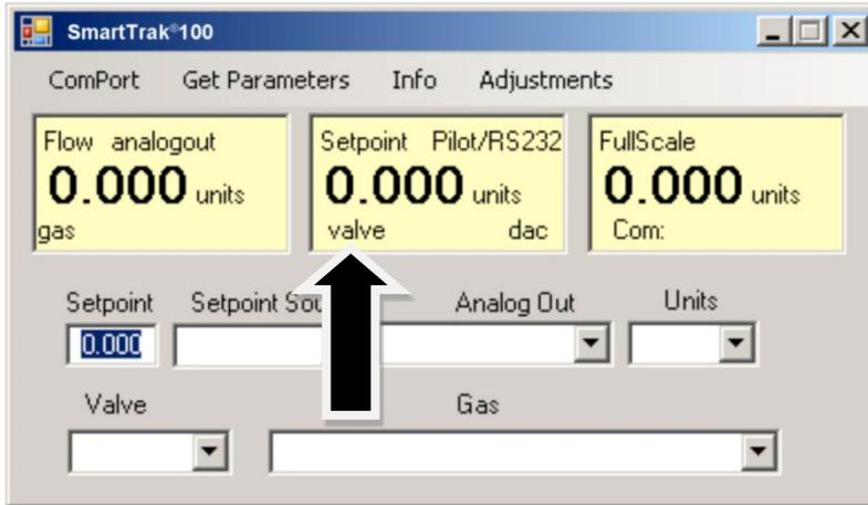
**If this box does not display “Automatic,” it will not be possible to control gas flow.** Your valve is locked open (Purge) or closed (Closed). See the section titled “Change Valve Operation” below for further instructions
