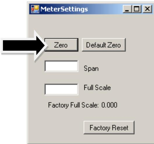
To perform this zero procedure, you must make sure that the actual flow is zero. Attempting to zero the meter or controller while there is a flow condition will cause an offset. Also, the best zero is obtained by using the actual gas at the listed operating pressure.
