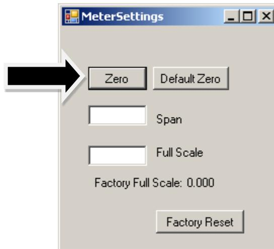
This screen allows for zeroing, spanning and adjusting the full scale for each of the 10 gases in the gas table individually. The screen will be displayed for the gas selected in the gas table on the main screen.
