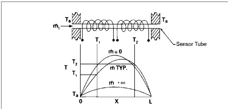
Figure 3. Sensor Temperature Distribution
