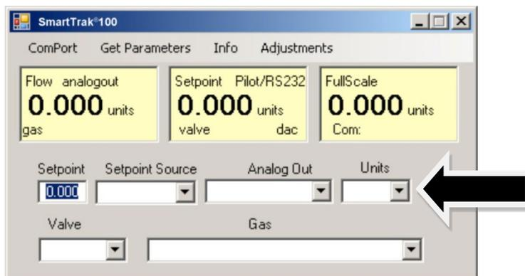
Make your selection, noting that each engineering unit is available with 3 different time constants: seconds, minutes and hours. Choose the combination of units and time constants you desire, then click. The box will display your new selection. Within a few seconds, the units will change in the Flow, Setpoint, and Full Scale boxes and the numerical values will be adjusted into the new units.
