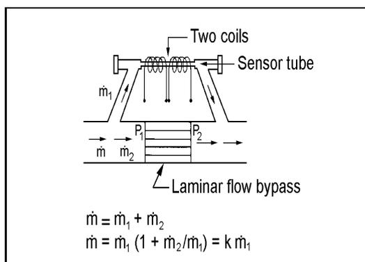
Figure 1. Flow Paths Through the Instrument.
