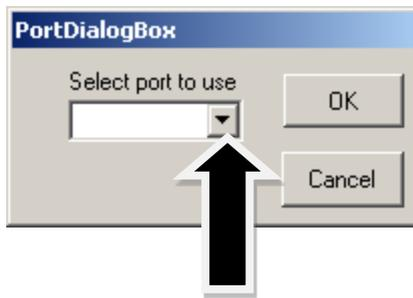
Use the pull-down menu to choose the port number that corresponds to the serial port channel your SmartTrak is connected to (from 1 to 255). If you have only one serial port, select “Comm Port 1.” When finished, click on the box marked “OK.”
