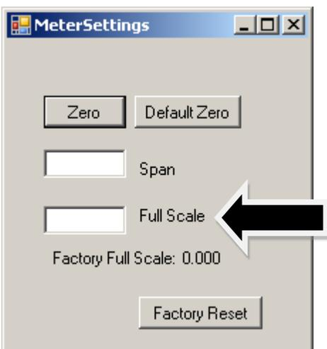
The instrument will display its current full-scale value. If your instrument is new or this value has never been modified, the value displayed will be 100% of the maximum flow rate your SmartTrak can measure or control without factory re-calibration. This is the number listed here:
