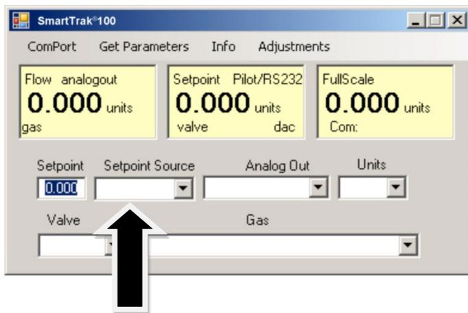
If, instead of using the RS-232 link, you prefer to supply analog set point signal to the SmartTrak, activate the pull-down menu. Make your selection carefully and click. Your selection will appear in the box and, after a few seconds, it will also appear in the yellow setpoint box.
