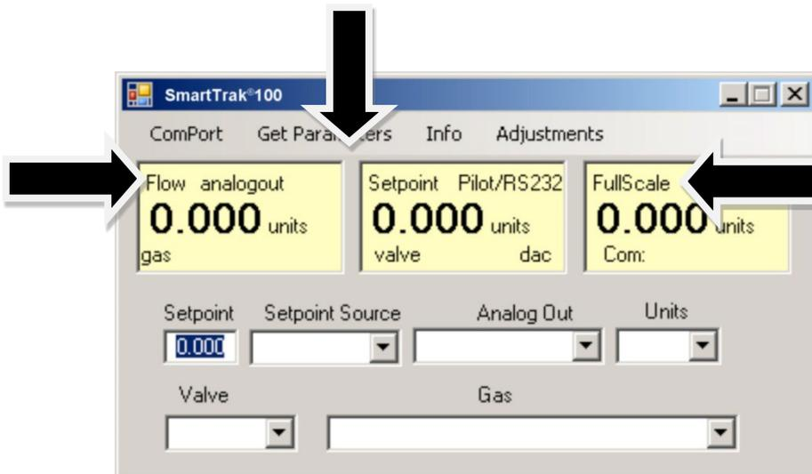
These boxes display the current operating conditions of your SmartTrak instrument. If you have the Pilot Module, these boxes on the upper half of the software screen are identical to the Upper Level Screens on the Pilot Module discussed in Chapter 4. The features of these boxes are described below.
