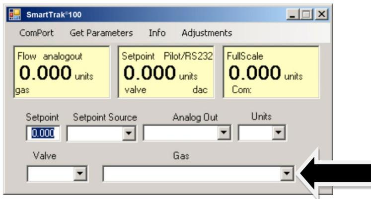
Choose the correct gas for your current application and click. The new gas selection will appear in the box. Within a few seconds, the new gas selection will also appear in the yellow Flow box and the values of the mass flow, setpoint and the full scale will be adjusted for this new gas. This is normal. In some cases, where the thermal properties of one gas are very similar to another, these values may not change very much.
