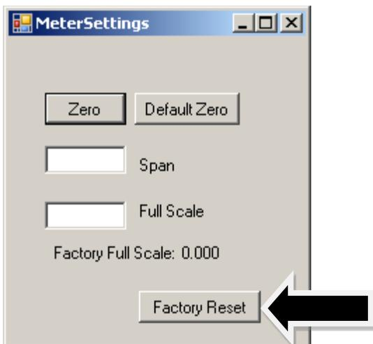
Here are some guidelines to remember if you choose to modify the Full Scale Value: Changing the full-scale value of the instrument does not affect the accuracy of the measurement. Instrument accuracy is a percentage of the original factory full-scale value
