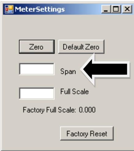
For example, the meter reads 98. The desired reading is 100. A span value of 1.02 will adjust the meter output to read 100.
