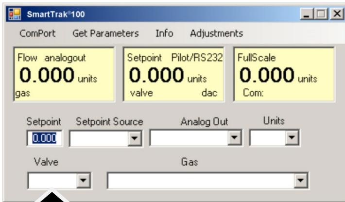
In this normal operating position, the valve is ready to control flow when it receives a setpoint from some source. Using this box, you may set the valve to open well beyond its normal maximum position (“Purge”) or force the valve to remain shut regardless of setpoint (“Closed”). Use the pull down menu to make this change. Choose “purge” to fully open the valve regardless of the given setpoint or choose “closed” to override any setpoint command and close the valve.
