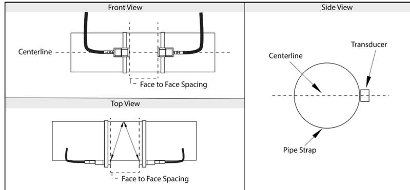
Figure 4. Transducer Spacing
