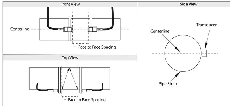
Figure 4. Transducer Spacing
