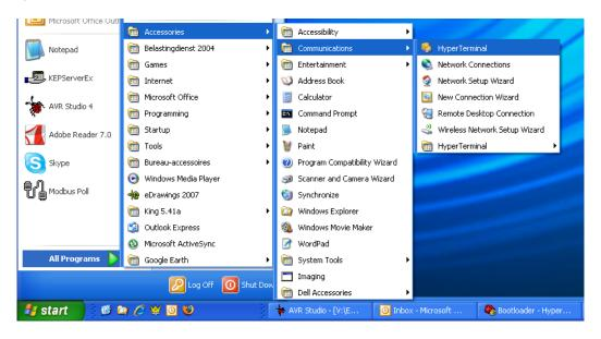
3. Start HyperTerminal from windows, and select the com port to which the RS-485 interface is connected. Use the following settings:
