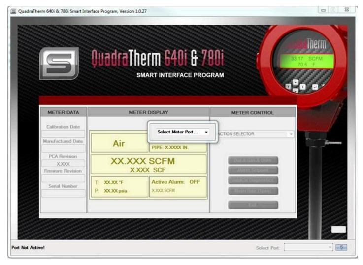
Step 8: Select the active port and all flow meter information will be read into the SIP application.
