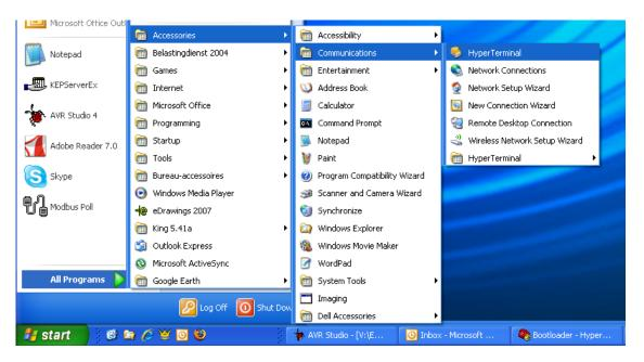
3. Start HyperTerminal from windows, and select the com port to which the RS-485 interface is connected. Use the following settings:
