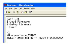
4. The screen will start to fill up with the "\seta" character indicating that the XMODEM transfer can be started. Press the "ESC" key to abort (if needed).
