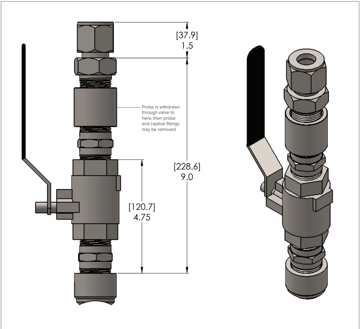
Side View-High Pressure Hot-Tap with Retractor to 400 psig (27.6 barg) (Model Code: L( )S9)
