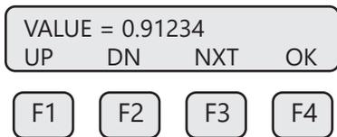
Press the **UP (F1)** or **DN (F2)** key to select a new digit or character, the cursor points to the selected digit. Press **NXT (F3)** to select the next digit and **OK (F4)** to accept the entry.
