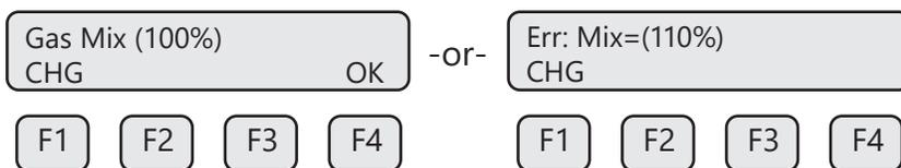
If the gas mix does not equal 100%, press **CHG (F1)** to return to the gas entry menu.
