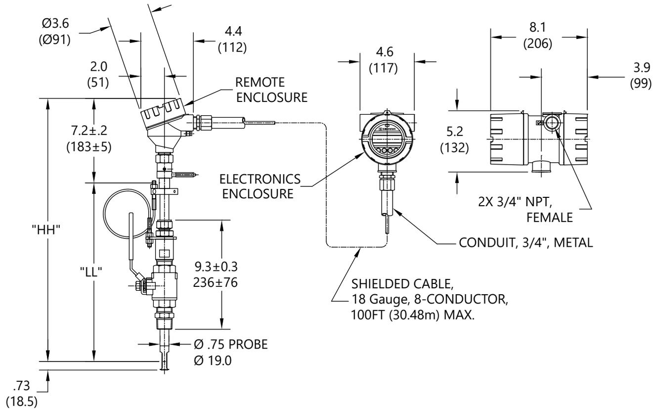
Table 7.2: Remote 645i Insertion Meter with Retractor
