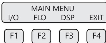
Then press **I/O (F1)** to set "Inputs/Outputs":
