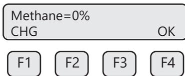
This screen shows the percentage of the gas mixture allocated to "Methane." In this case, it shows 0%. To program the specific mixture of "Methane", press **CHG (F1)**.
