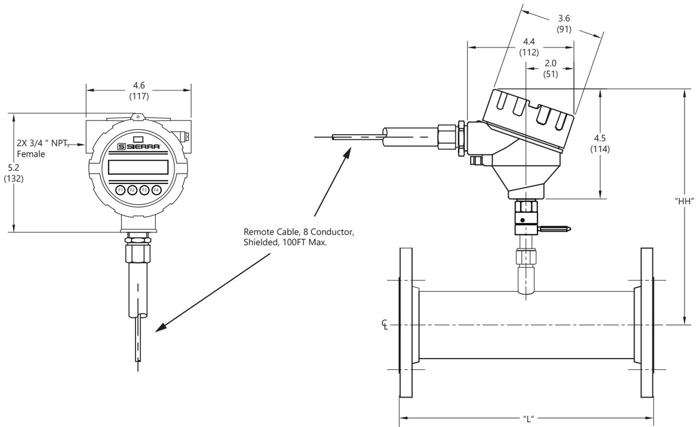
Table 7.9: 745i Inline Remote Meter with 316 Stainless Steel Flow Body and 150 lb RF Flange End Connections Dimensions
