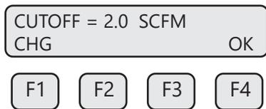
Enter the value for the flow cutoff and then press **OK (F4)**. When the flow rate falls below the flow cutoff, the flow meter will display a flow value of zero.
