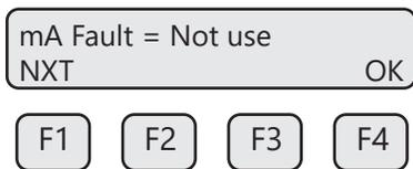
This menu allows the user to select an alarm fault level on the 4-20mA output. The alarm is activated when a serious issue is detected preventing the calculation of the correct flow rate. The 3.6mA and 21mA alarm outputs are related to the NAMUR NE 43 alarm feature.
