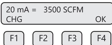
Enter the value for the 20mA and press **OK (F4)** key to accept the setting. Then the following screen will display:
