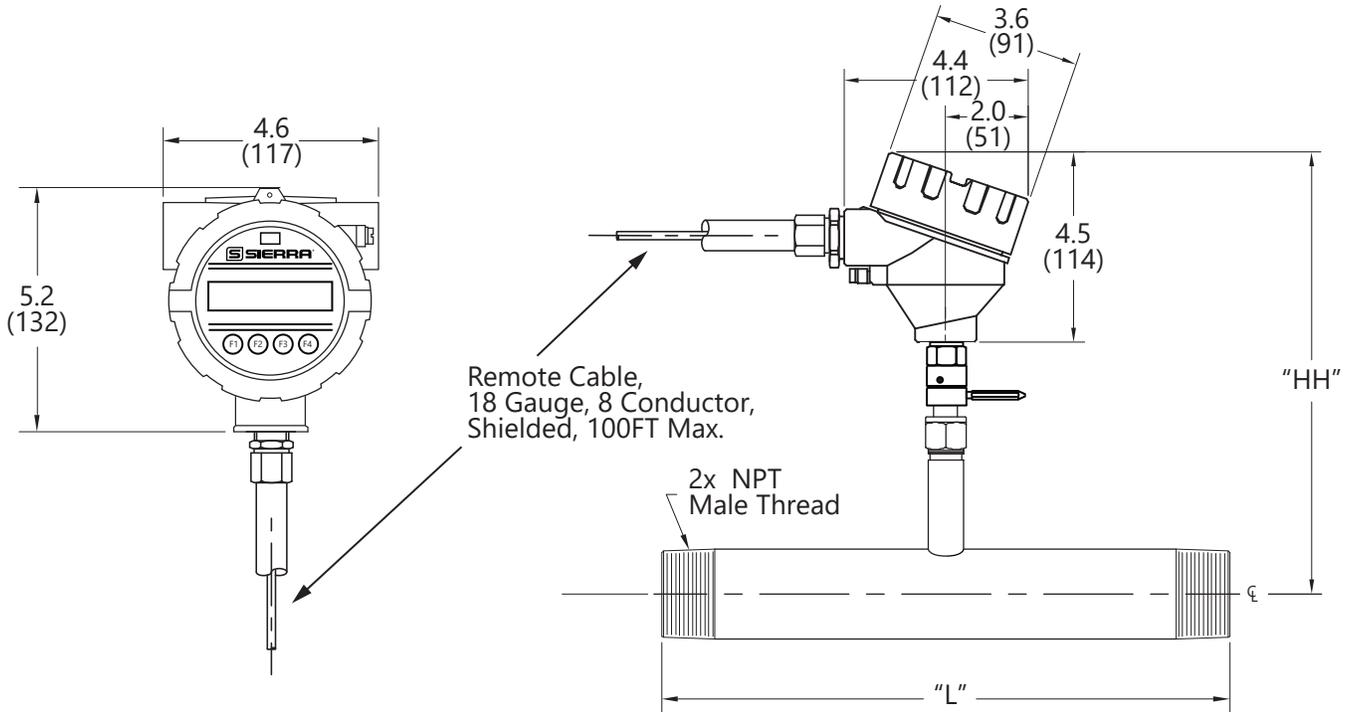
Table 7.7: 745i Inline Remote Meter with 316 Stainless Steel Flow Body and NPT End Connections
