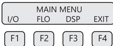
This is the "Main Menu" for the programming mode. To exit the programming mode, press **EXIT (F4)** repeatedly until "Normal Mode" is seen briefly. Choose **I/O (F1)** to access the communication output.
