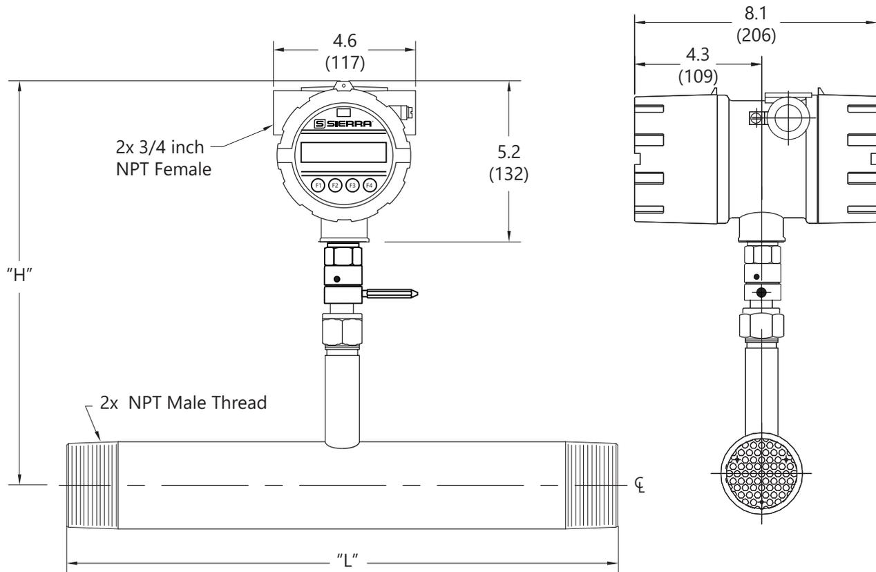
Table 7.6: 745i Inline Meter with 316 Stainless Steel Flow Body and NPT End Connections
