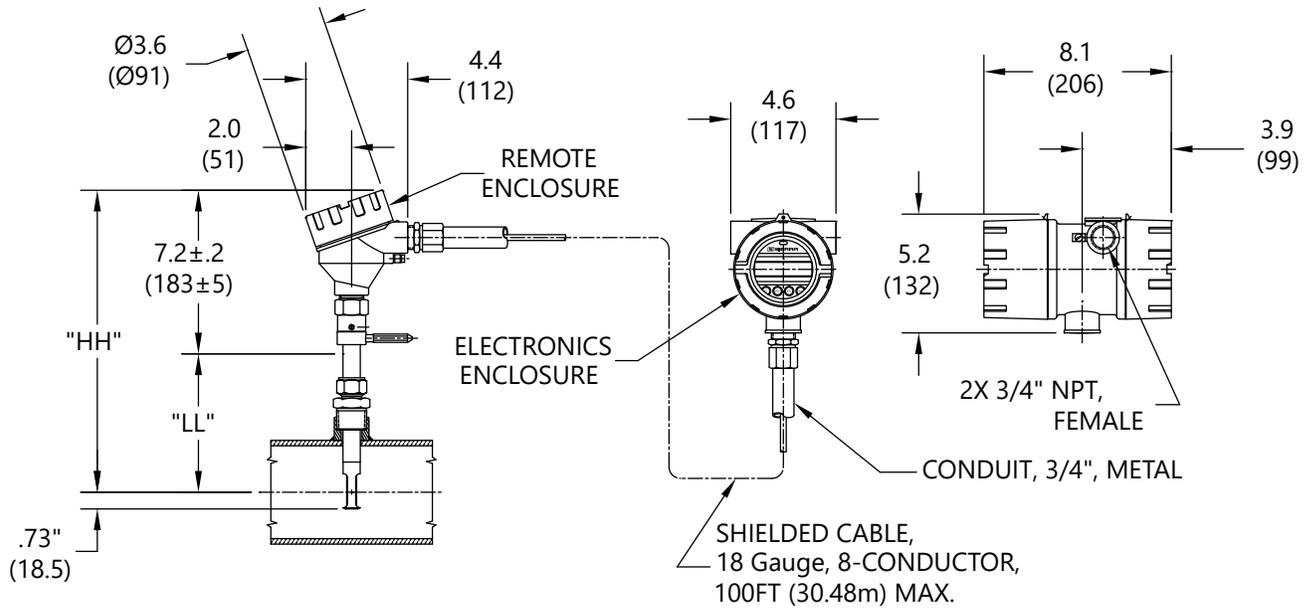
Table 7.5: 645i Insertion Remote Meter with 316 stainless steel probe
