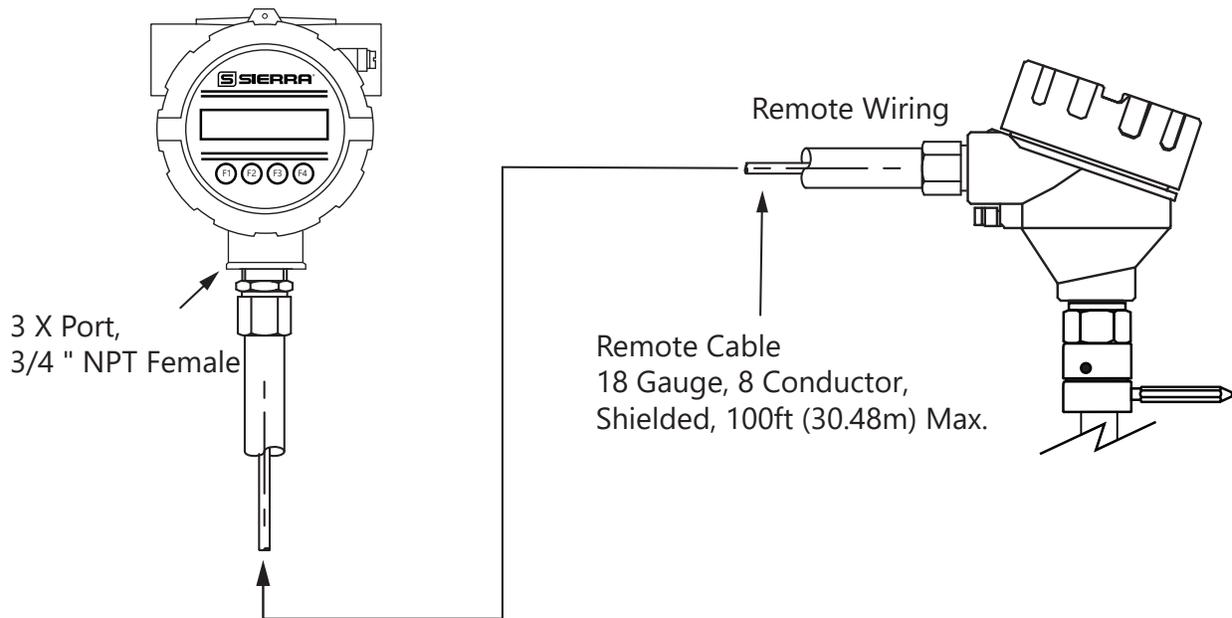
Use an extension cable to connect the 645i/745i remote sensor to the electronics enclosure.
