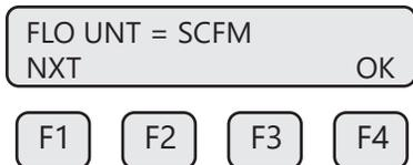
Press **NXT (F1)** key repeatedly until the correct selection is made and **OK (F4)** key to accept the entry.
