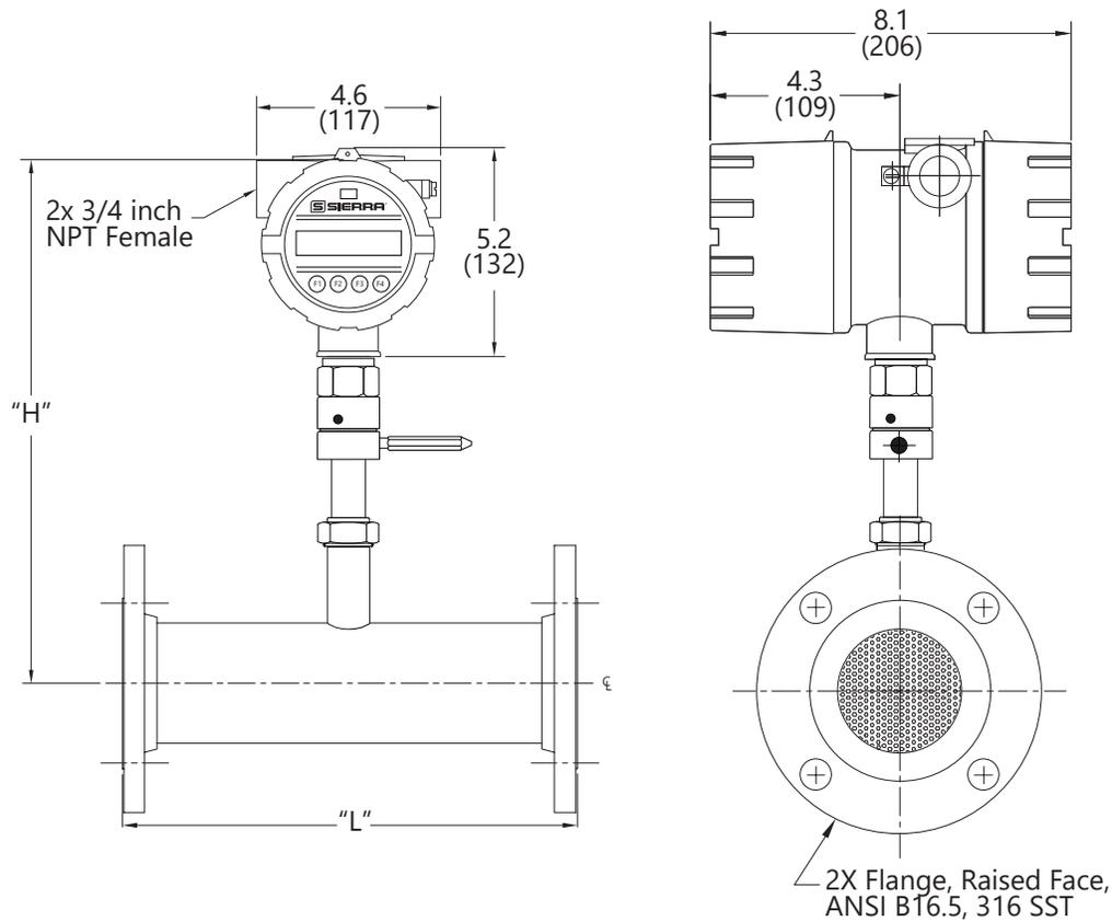
Table 7.8: 745i Inline Meter with 316 Stainless Steel Flow Body and 150 lb RF Flange End Connections Dimensions
