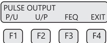
Use **P/U (F1)** to enter pulse per unit, **U/P (F2)** for unit per pulse or **FEQ (F3)** to enter the flow and maximum frequency to scale the pulse/alarm output.
