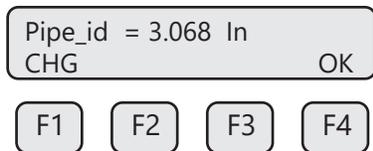
Use millimeters for metric flow unit selections and inches for English flow unit selections. This selection is dependent on the flow unit selected (English vs metric). If the pipe/duct is a square or rectangle, the hydraulic diameter (equivalent value for a round pipe) must be entered for the pipe ID.
