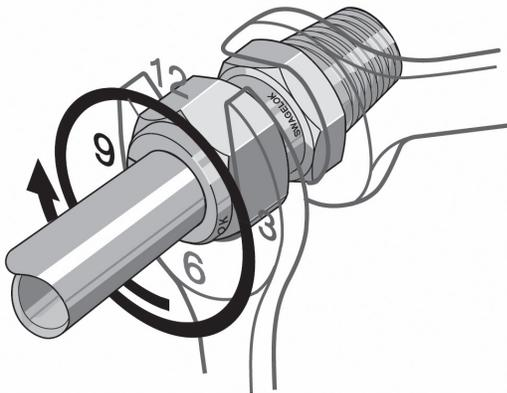
**NOTE!** Before removing a probe with compression fitting, mark the tube at the back of the nut, and mark a line along the nut and fitting body. Use these marks when reinstalling the probe. Reference the instructions on p. 28.
