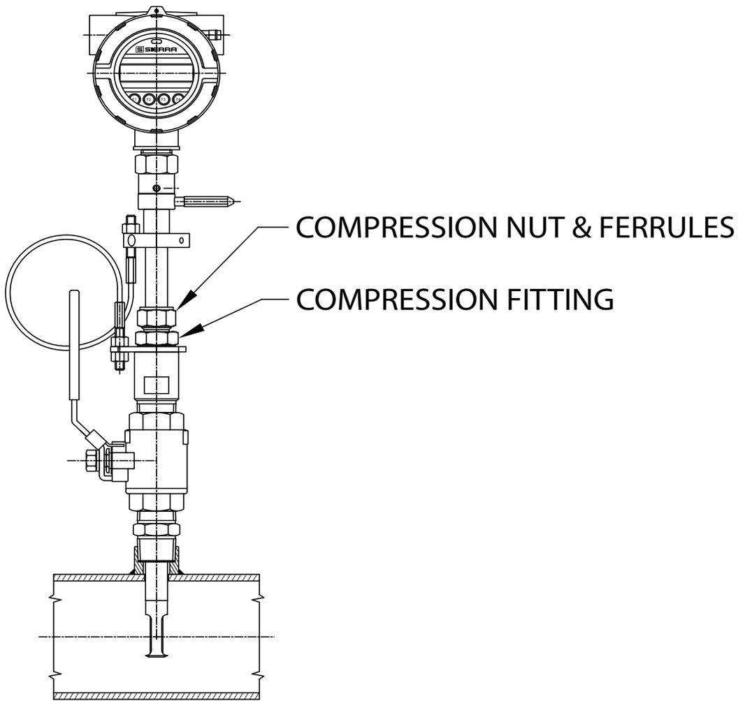
5. Secure the probe in place by tightening the compression nut with a 1 1/8" wrench and a 1 1/4" wrench on the compression fitting. See p. 27 of the manual for detailed instructions to tighten the compression nut.
