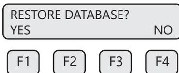
Press **YES (F1)** ONLY if you want to restore your database to the initial factory setting that the meter was shipped with. All current user-entered settings will be overwritten. The green LP3 LED will flash at a faster pace until the recall is performed. The "RESET CRC" screen will follow "RESTORE DATABASE". Upon pressing **OK (F4)**, an option to reset the NVRAM CRC will follow.
