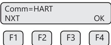
Press **NXT (F1)** until HART is selected as shown and then press **OK (F4)** to accept the setting.
