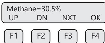
To set the percentage of "Methane" in the gas mix, press **UP (F1)** or **DN (F2)** to choose the first digit of the percentage. Press **NXT (F3)** to move to the next digit in the percentage and then use **UP (F1)** or **DN (F2)** again to choose the next digit of the percentage. Once the desired "Methane" percentage is displayed, press **OK (F4)**. the display will move to view the concentration of Carbon Dioxide.
