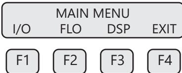
This is the "Main Menu" screen for the programming mode. To exit the programming mode, press **EXIT (F4)** repeatedly until "Normal Mode" is briefly displayed.
