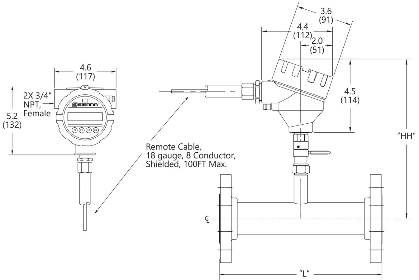
Table 7.11: 745i Inline Remote Meter with 316 Stainless Steel Flow Body and 300 lb RF Flange End Connections Dimensions
