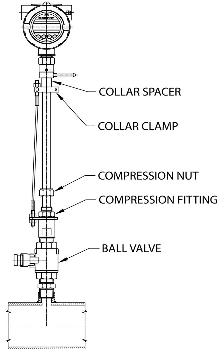
**i NOTE!** At a maximum system pressure of 150 psig, the force required to push the probe in place to tighten the compression Nut will be approximately 66 lbs.
