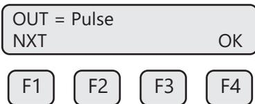
Press **NEXT (F1)** to cycle through output options until you have the selection for "OUT=Pulse" and press **OK (F4)**.
