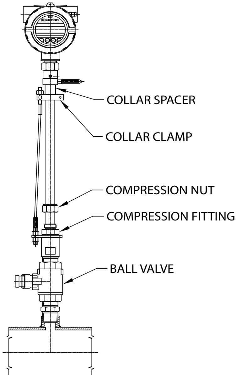
**How to Insert the Probe into the Flow Stream (Valve closed, System Pressurized)**
