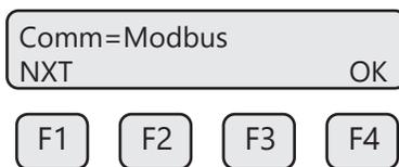
Press **NXT (F1)** repeatedly until Modbus is selected as shown and then press **OK (F4)** to accept the setting.
