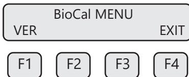
Press **VER (F1)** to perform the BioCal™ verification test.
