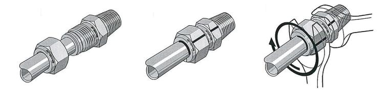
**CAUTION!** Do not use a gap inspection gauge with reassembled fittings.
