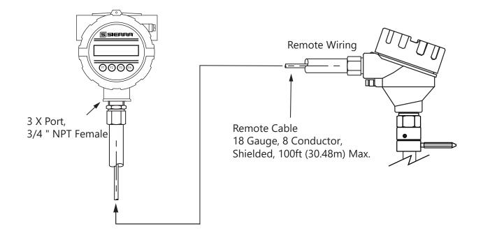
Use an extension cable to connect the 645i/745i remote sensor to the electronics enclosure.
