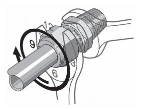
**NOTE!** Before removing a probe with compression fitting, mark the tube at the back of the nut, and mark a line along the nut and fitting body. Use these marks when
