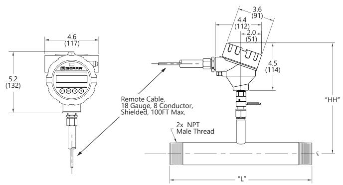
Fig 7.7: 745i Inline Remote Meter with 316 Stainless Steel Flow Body and NPT End Connections Dimensions
