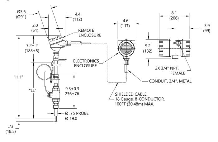
*Fig. 7.2: Remote 645i Insertion Meter with Retractor Dimensions*
