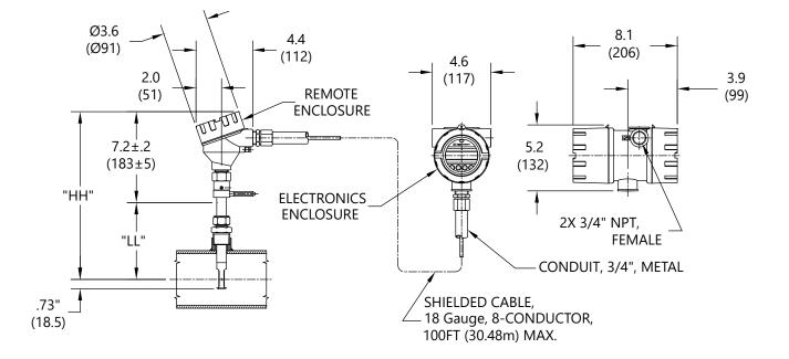
Table 7.5: 645i Insertion Remote Meter with 316 stainless steel probe
