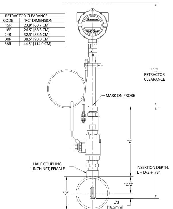
Fig. 2.12: Determining and Marking Insertion Depth
