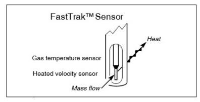
Figure 1. 730 FastTrak Sensor Probe
