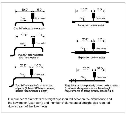
Figure 2. Recommended Pipe Length Requirements for Installation
