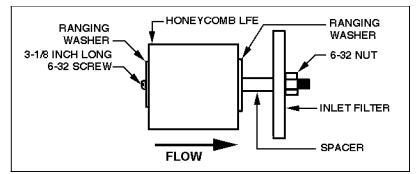
Figure 4-6. High Flow Transducer LFE Cleaning
