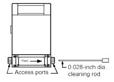
2. Flush the sensor tube with a non-residuous solvent compatible with the O-ring material. In cases where solids are deposited in sensor, units should be returned to factory for complete cleaning and re-calibration.
