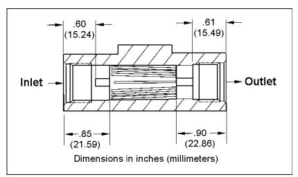
Figure 4-2. Correct LFE Position
