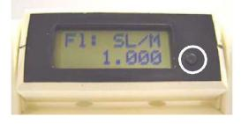
Screen 1 (start-up screen shown in photo above): Flow units are shown together with the actual flow
