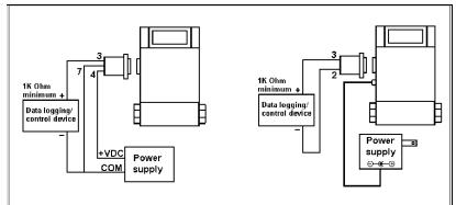
Figure 2-3. Standard 0-5 VDC Output Signal Wiring
