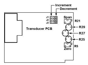
Figure 4-7. Printed Circuit Board Component Locations
