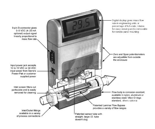
Figure 1-1. Top-Trak Features (Typical)
