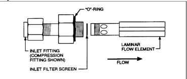
Figure 4-4. Low Flow Transducer LFE Cleaning
