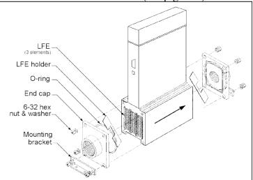
Figure 4-3. Model 826/827 Flow Components
