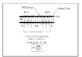
Figure 1-3. Flow Measuring Principle
