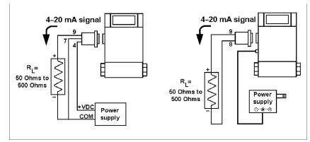
Figure 2-4. Single Transducer Current Loop Connection
