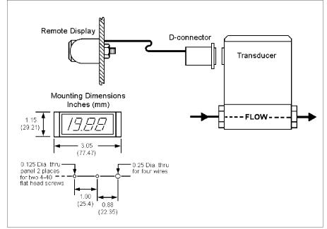
Figure 2-6. Mounting the Remote Display
