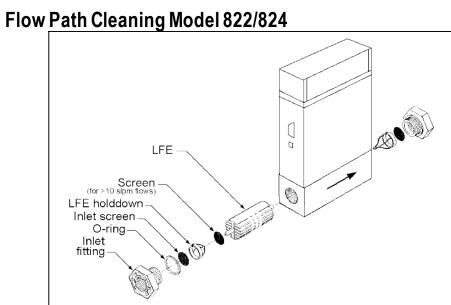
Figure 4-1. Model 822/824 Flow Components
