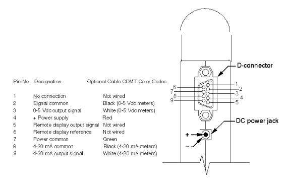
Figure 2-2. Transducer D-Connector Pin Assignments
