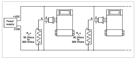
Figure 2-5. Multiple Transducer Current Loop Connections
