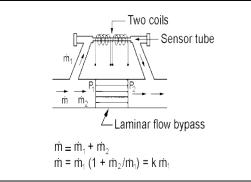
Figure 1-2. Flow Paths through the Transducer
