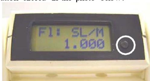
**Screen 1** (start-up screen shown in photo above): Flow units are shown together with the actual flow
