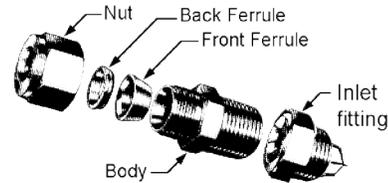
3. **Hold the body steady with a backup wrench.** For 1/2-inch size, tighten the nut 1-1/4 turns from finger tight. For 1/8-inch, 1/4-inch and 3/8-inch sizes, tighten only 3/4 turn from finger tight. **Do not over-tighten!**
