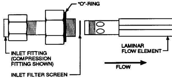
Figure 4-1. Low Flow Transducer LFE Cleaning
