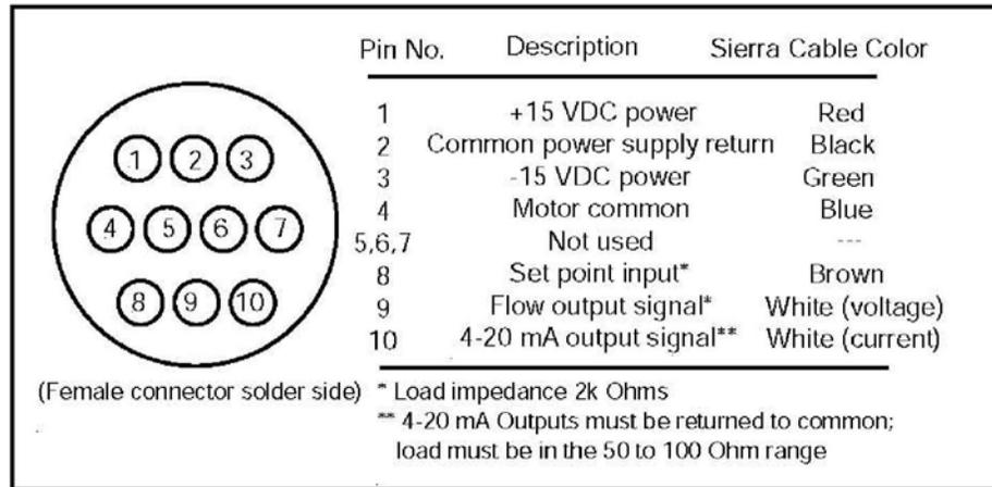
Figure 2-16. Motor-Operated Rotary Valve Connector (10-Pin Connector)
