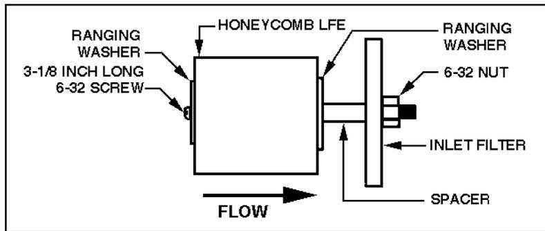
Figure 4-3. High Flow Transducer LFE Cleaning
