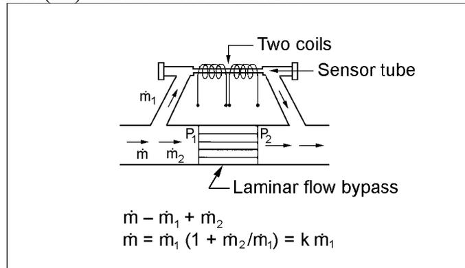
Figure 1-1. Flow Paths through the Transducer
