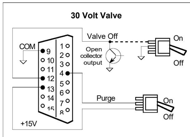
Figure 2-14. Valve Purge and Valve Off (15-Pin D-Connector)
