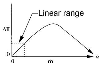
Figure 1-4. Linear Range of the Transducer's Output Signal
