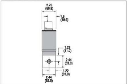
Shaded portion of dimensional drawings indicates 840 controllers.
