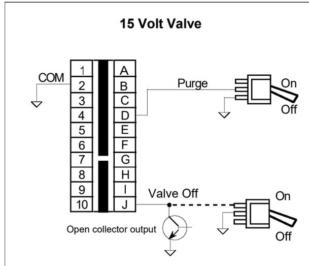
*Valve Purge and Valve Off (20-Pin Connector)*
