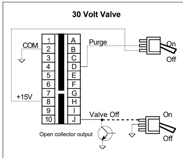
Note: Typically controllers for 10 slpm or below will be equipped with a 15-volt valve circuit, while those above 10 slpm with a 30-volt circuit. Consult Technical Support if necessary.
