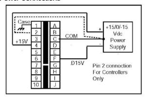
Figure 2-2. Input Power Connections (20-Pin Connector)
