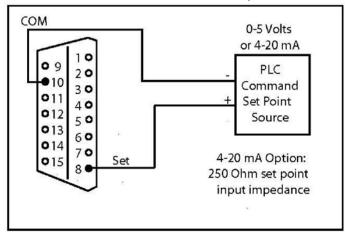
Figure 2-12. External Command Set Point Source (1 5-Pin D-Connector)
