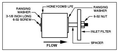
Figure 4-3. High Flow Transducer LFE Cleaning
