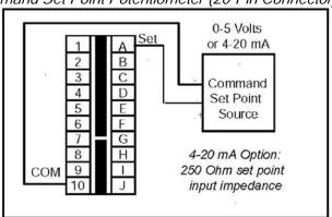
Figure 2-5. External Command Set Point Source (20-Pin Connector)
