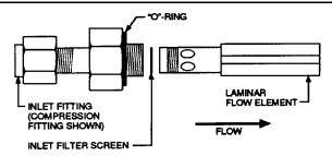
Figure 4-1. Low Flow Transducer LFE Cleaning
