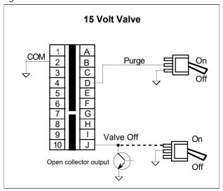
Valve Purge and Valve Off (20-Pin Connector)
