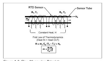
Figure 1-2. Flow Measuring Principle
