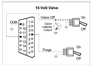
Figure 2-13. Valve Purge and Valve Off (15-Pin D-Connector)
