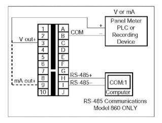
Figure 2-3. Output Signal Connections (20-Pin Connector)
