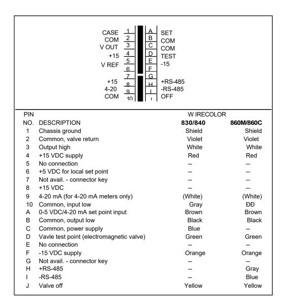
Figure 2-8.20-Pin Connector Pin Designations
