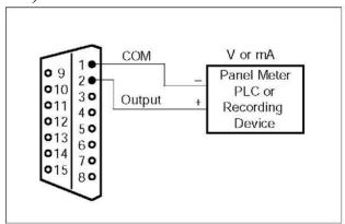
Figure 2-10. Output Signal (15-Pin D-Connector)
