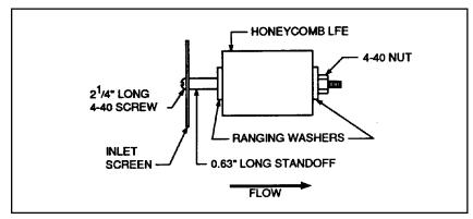
Figure 4-2. Medium Flow Transducer LFE Cleaning
