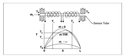
Figure 1-3. Sensor Temperature Distribution
