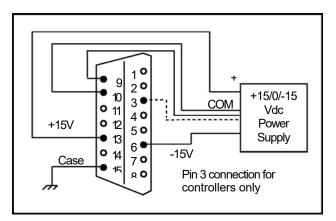
Figured 2-9. Input Power (15-Pin D-Connector)
