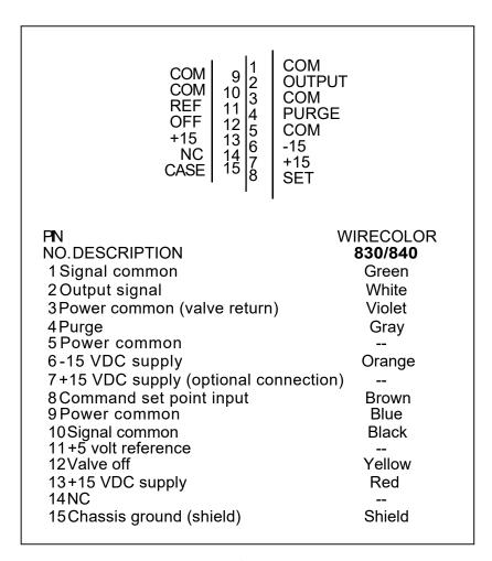
Figure 2-15. 15-Pin D-Connector Pin Assignments
