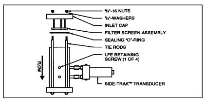
Figure 4-4. NPT Transducer LFE Cleaning
