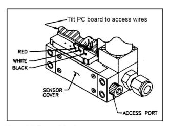
Figure 4-5. Sensor Wire Access
