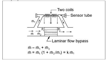
Figure 1-1. Flow Paths through the Transducer
