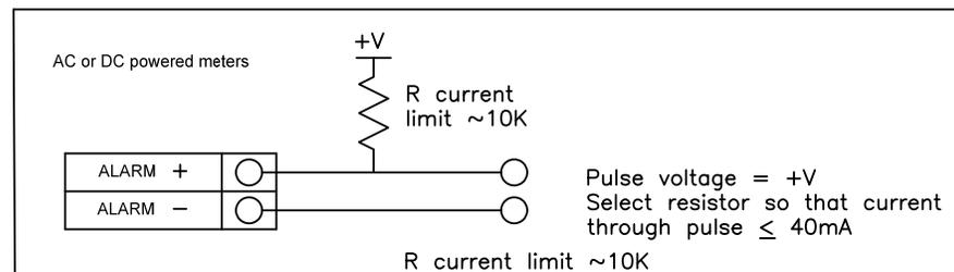
Figure 2-33. Isolated Alarm Output with External Power Supply
