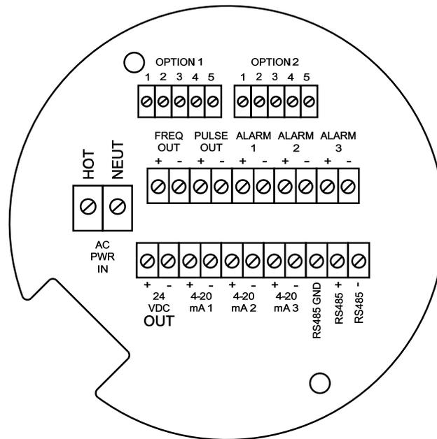
Figure 2-22. AC Wiring Terminals
