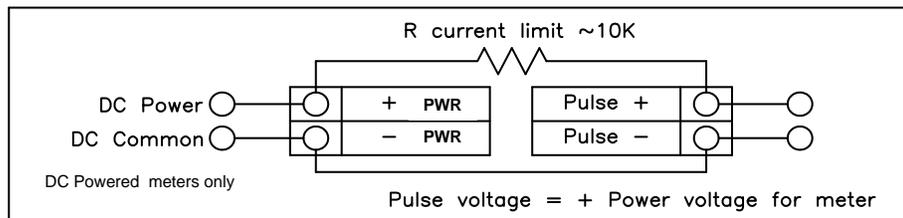
Figure 2-31. Non-Isolated Pulse Output Using Input Power Supply
