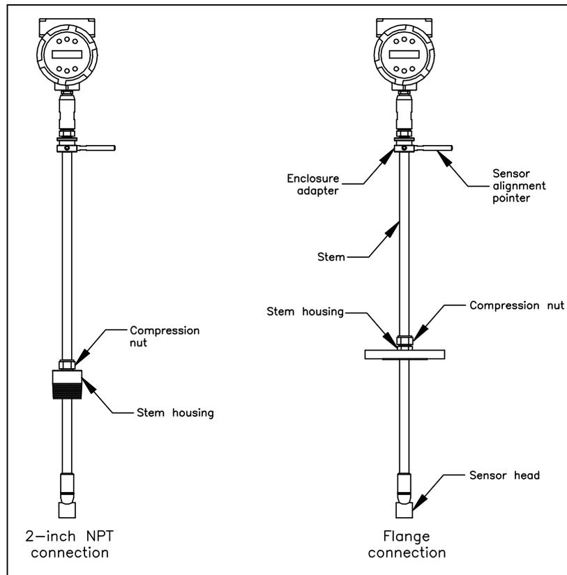
Figure 2-7. Flow Meter with Compression Type Fitting
