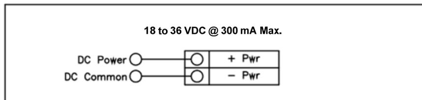
Figure 2-25. DC Power Connections
