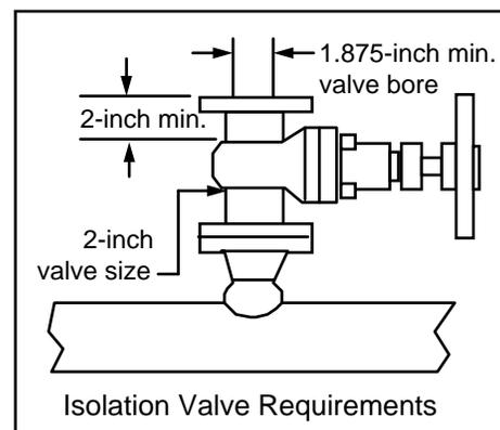
3. Choose an isolation valve with at least two inches existing between the flange face and the gate portion of the valve. This ensures that the flow meter's sensor head will not interfere with the operation of the isolation valve.
