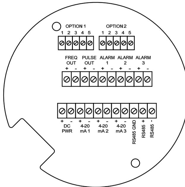
Figure 2-24. DC Wiring Terminals
