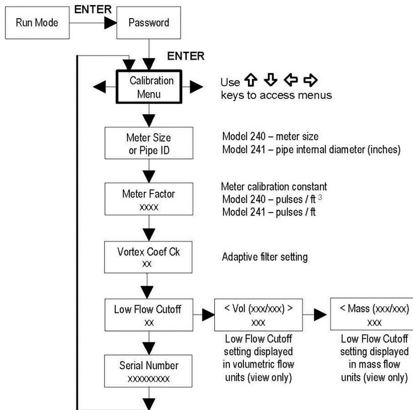
The Calibration Menu contains the calibration coefficients for the flow meter. These values should be changed only by properly trained personnel. The Vortex Coef Ck and Low Flow Cutoff are set at the factory. Consult the factory for help with these settings if the meter is showing erratic flow rate.
