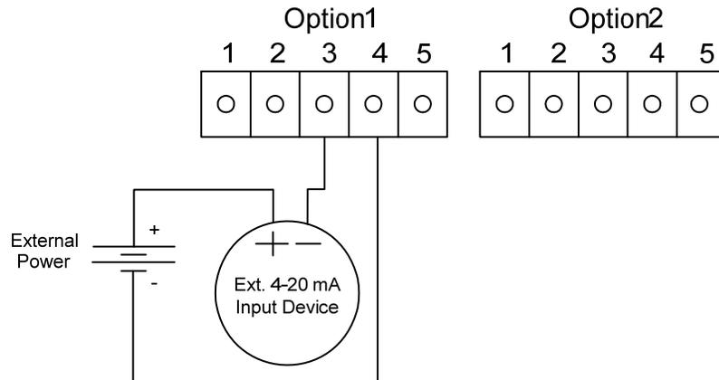
Figure 2-38. External 4-20 mA Input Wiring - External Power Supply
