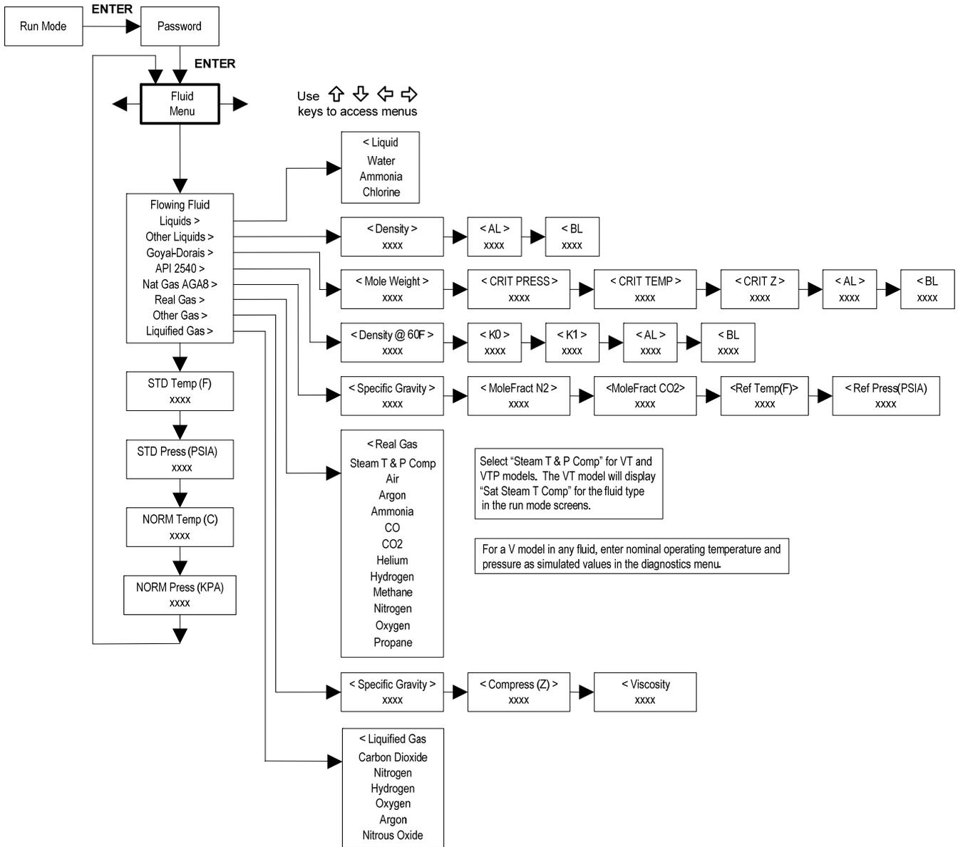
Use the Fluid Menu to configure the flow meter for use with common gases, liquids and steam. Your flow meter is pre-programmed at the factory for your application's process fluid.
