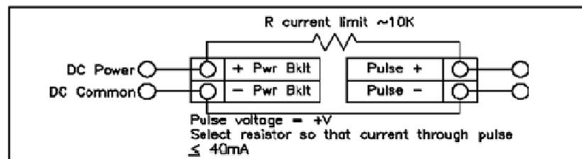
Figure 2-18. Non-Isolated Pulse Output Using External Power Supply
