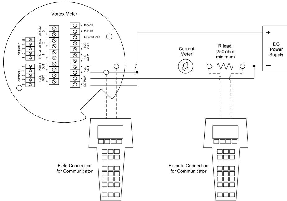
Figure 4-2. DC Powered Meter Wiring (HART)
