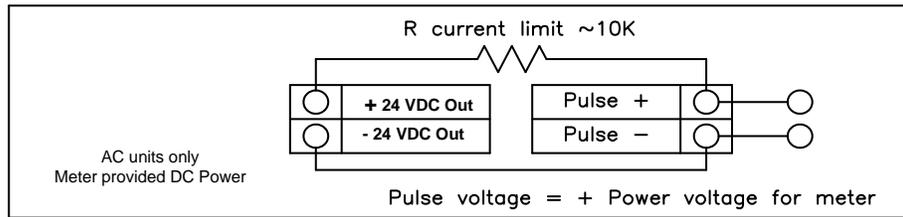
Figure 2-32. Isolated Pulse Output Using Meter Provided Power Supply
