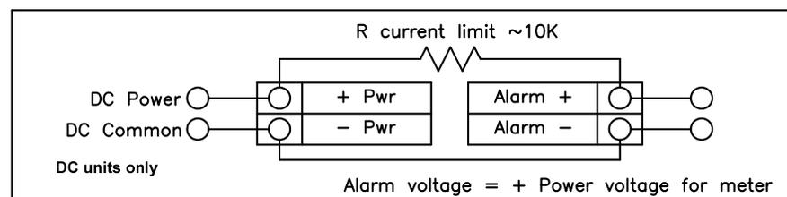
Figure 2-34. Non-Isolated Alarm Output Using Internal Power Supply
