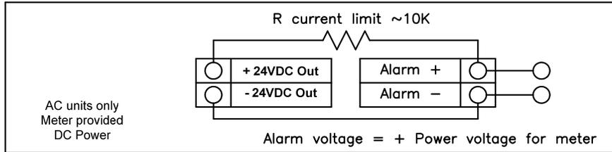
Figure 2-35. Isolated Alarm Output Using Meter Provided Power Supply
