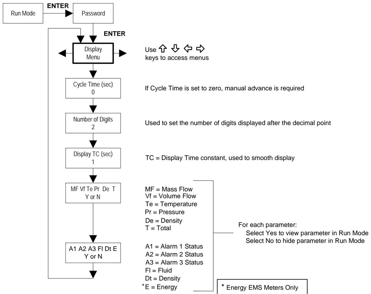
Use the Display Menu to set the cycle time for automatic screen sequencing used in the Run Mode, change the precision of displayed values, smooth the values or enable or disable each item displayed in the Run Mode screens.
