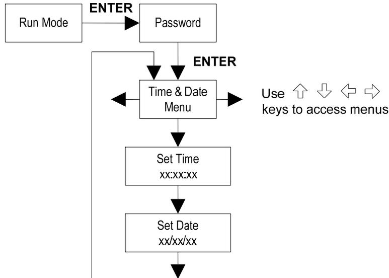
Use the Time and Date Menu to enter the correct time and date into the flow meter's memory. The parameters are used in the Run Mode and the alarm and system log files.
