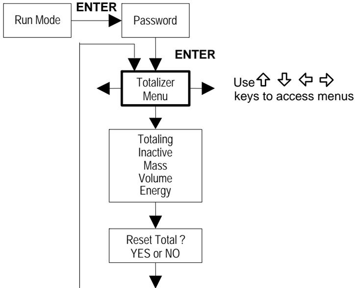
Use the Totalizer #2 to Monitor Flow or Energy. Note that Totalizer #2 does not operate a relay, it is for monitoring only.
