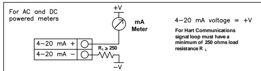
Figure 2-27. Isolated 4-20 mA Output with External Power Supply
