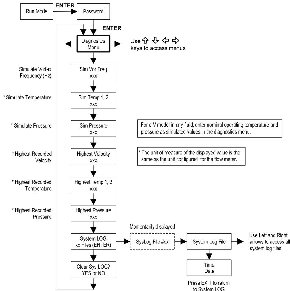
Use the Diagnostics Menu to simulate operation and review the system files. The system log files contain time/date stamped messages including: power on, power off, programming time outs, parameter faults, incorrect password entry and other various information relative to system operation and programming.
