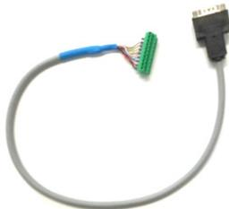
**Note:** Since the **housing is open** for operation, this type of communication **cannot** be used under IP67/Ex conditions. The IAC cable is not approved for ATEX or IP67 and is **not designed for permanent use**.
