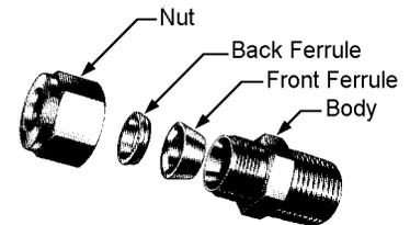
Follow the installation instructions that are applicable to your instrument's process connection. Ensure that the tubing is free from burrs or sharp rims that may result from cutting.
