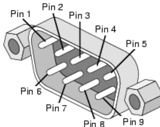
*DB9 Pin-out locations on instrument. There are two DB9 connectors, one on each side of the enclosure. Assure block off plate covers unused DB9...*
