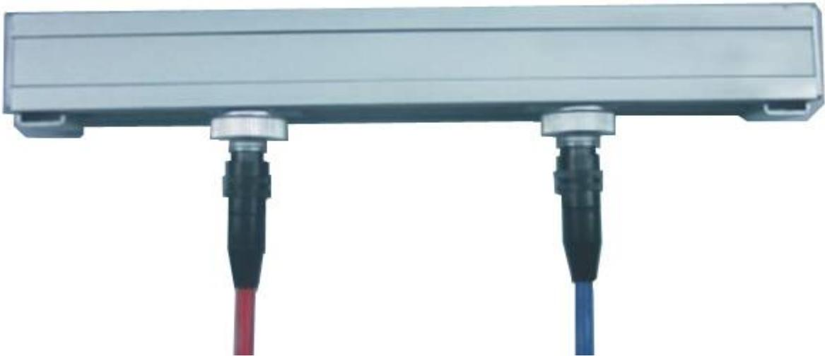
When finished installing both transducers in a single rack, they should appear as shown in the photo below. The oval transducer crystals should be facing each other. They are designed to send signals back and forth to one another, and if they are installed backwards, they will not function.
