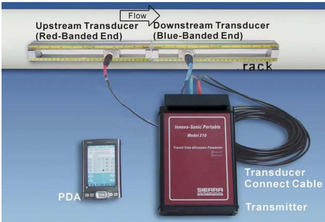
When installing transducers to relatively small pipes {sizes under 8” in most applications}, the transducer spacing displayed in MENU25 may be less than 7.5” (190mm), then we can install the transducers in single slide ruler rack. The installation method is unscrewing a transducer off the rack at first,
