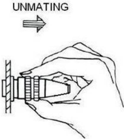
UNMATING: As drawing shows, hold the coupling nut and pull to unmate.
