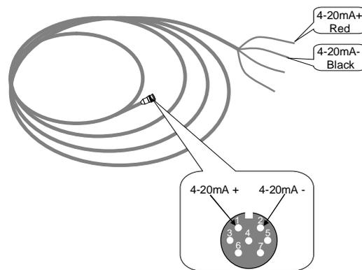
The 4~20mA current output connects to the 7-pin din jack on the panel. The color of cable core is red (4-20mA+) and black (4-20mA-). With an accuracy of 0.1%, The current output of the 210 PORTABLE is fully programmable and can be set to various output modes such as 4~20mA or 0~20mA. Use Window M55 to select the output mode.
