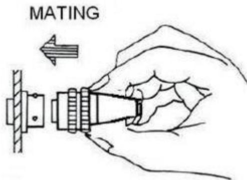
**MATING:** As drawing shows, hold the smooth part in back of the plug and push when the key of the plug are in line. The connector is fully seated when a click is heard or felt from the quick disconnect ring.
