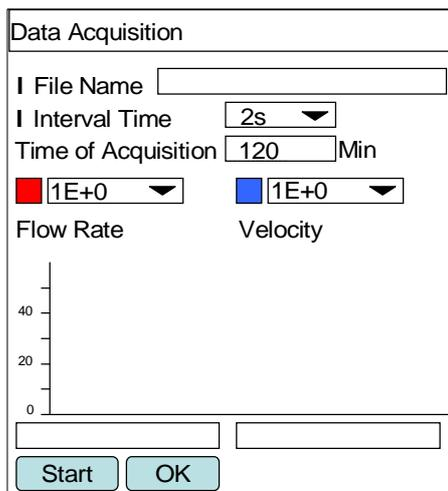
**File Name:** Give a name for the collected data. Input the name above the line manually, otherwise the name will be generated automatically.
