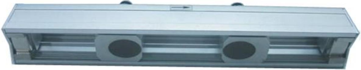
The flow meter will now work as usual. Exercise caution during this procedure as the transducers are spring loaded in the racks.
