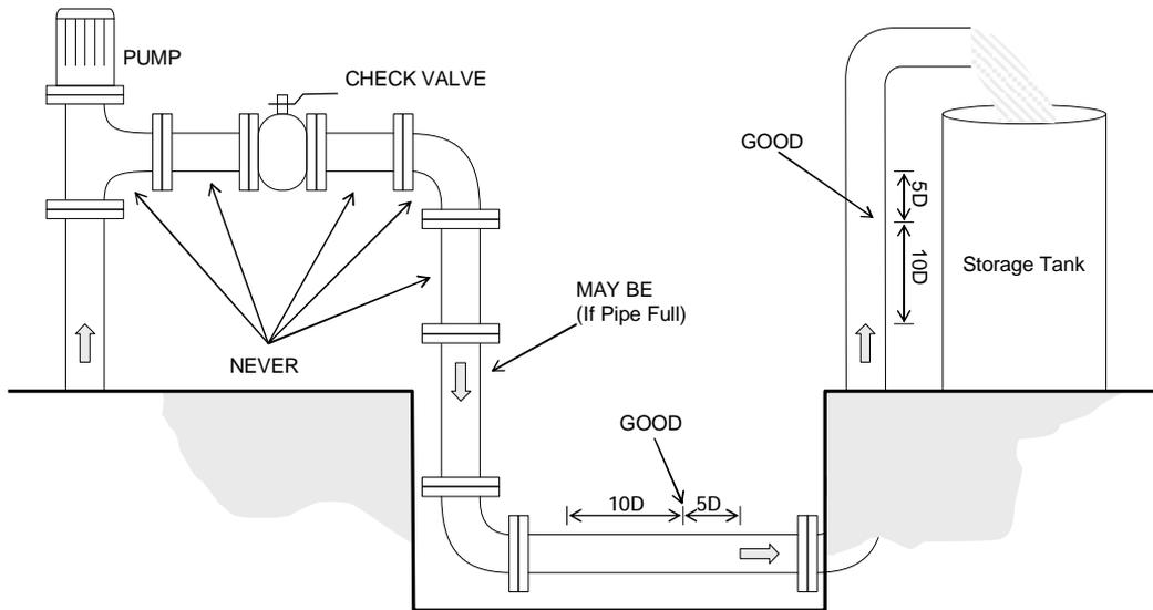
The site should have a straight pipe run length equal to at least 10 pipe diameters upstream and 5 pipe diameters downstream from any throttling valves or other flow disturbance producing elements, such as pipe reducers, elbows, tees, etc.
