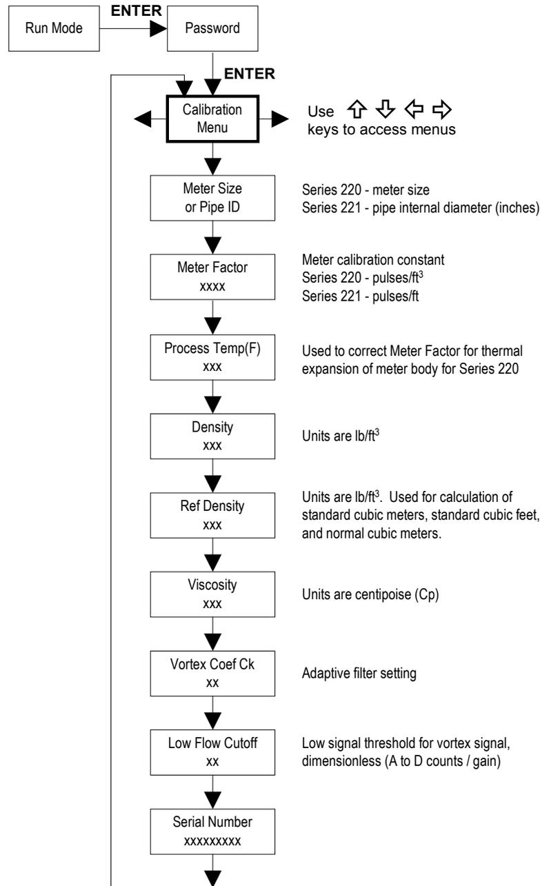
The Calibration Menu contains the calibration coefficients for the flow meter. These values should be changed only by properly trained personnel. The Vortex Coef Ck and Low Flow Cutoff are set at the factory. Consult the factory for help with these settings if the meter is showing erratic flow rate. The units of measurement used in the Calibration Menu are preset and are as follows: Density = lbm/ft<sup>3</sup>, Reference Density = lbm/ft<sup>3</sup>, Viscosity = centipoise.
