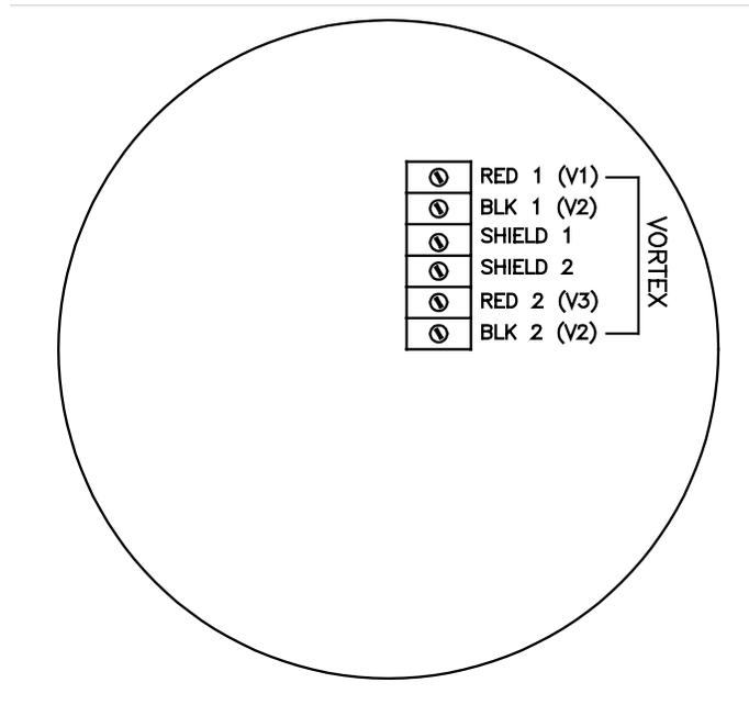
Figure 2-17. Junction Box Sensor Connections
