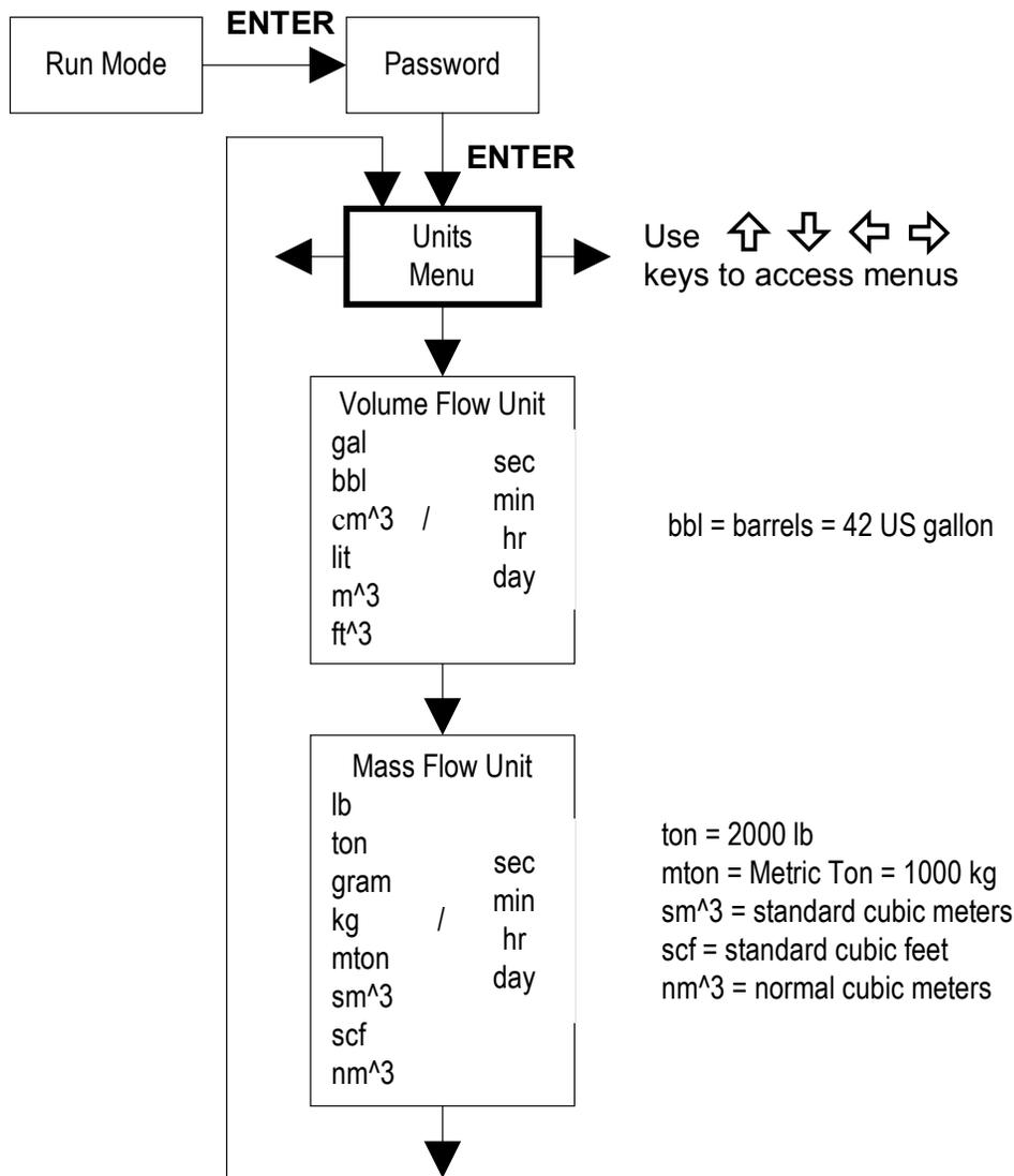
Use the Units Menu to configure the flow meter with the desired units of measurement. (These are global settings and determine what appears on all screens.)
