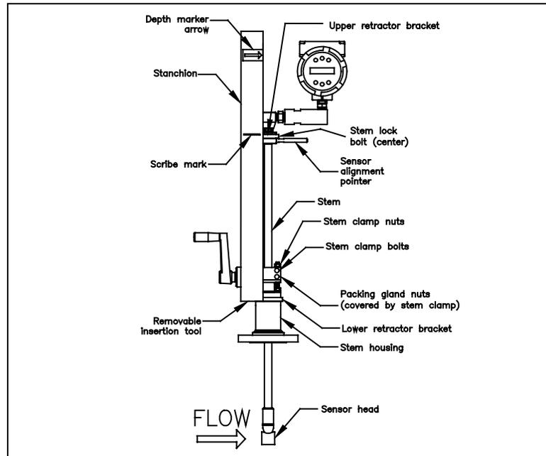
Figure 2-10. Flow Meter with Removable Insertion Tool
