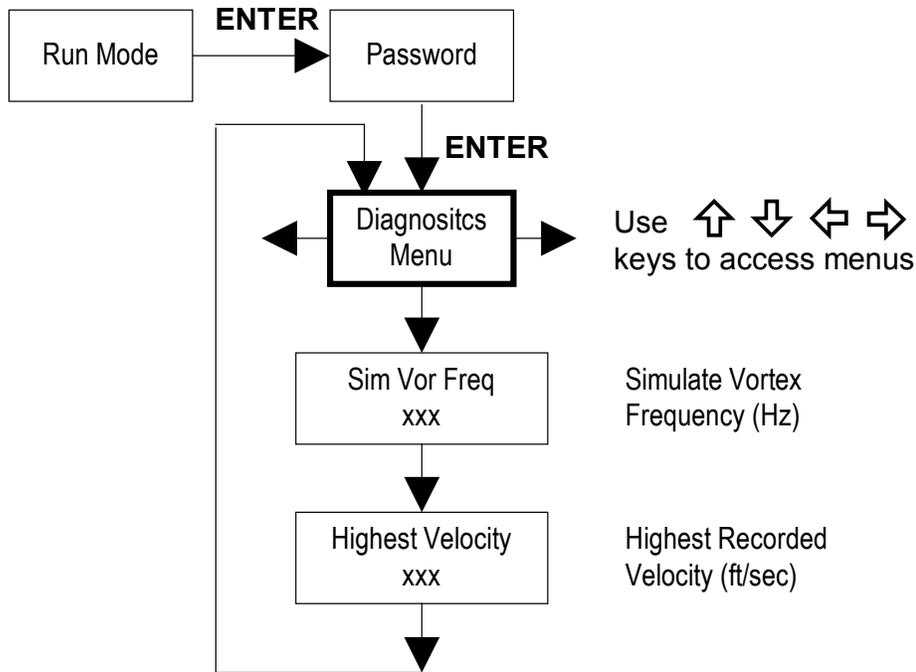
Use the Diagnostics Menu to simulate flow and review the highest recorded velocity in ft/sec.
