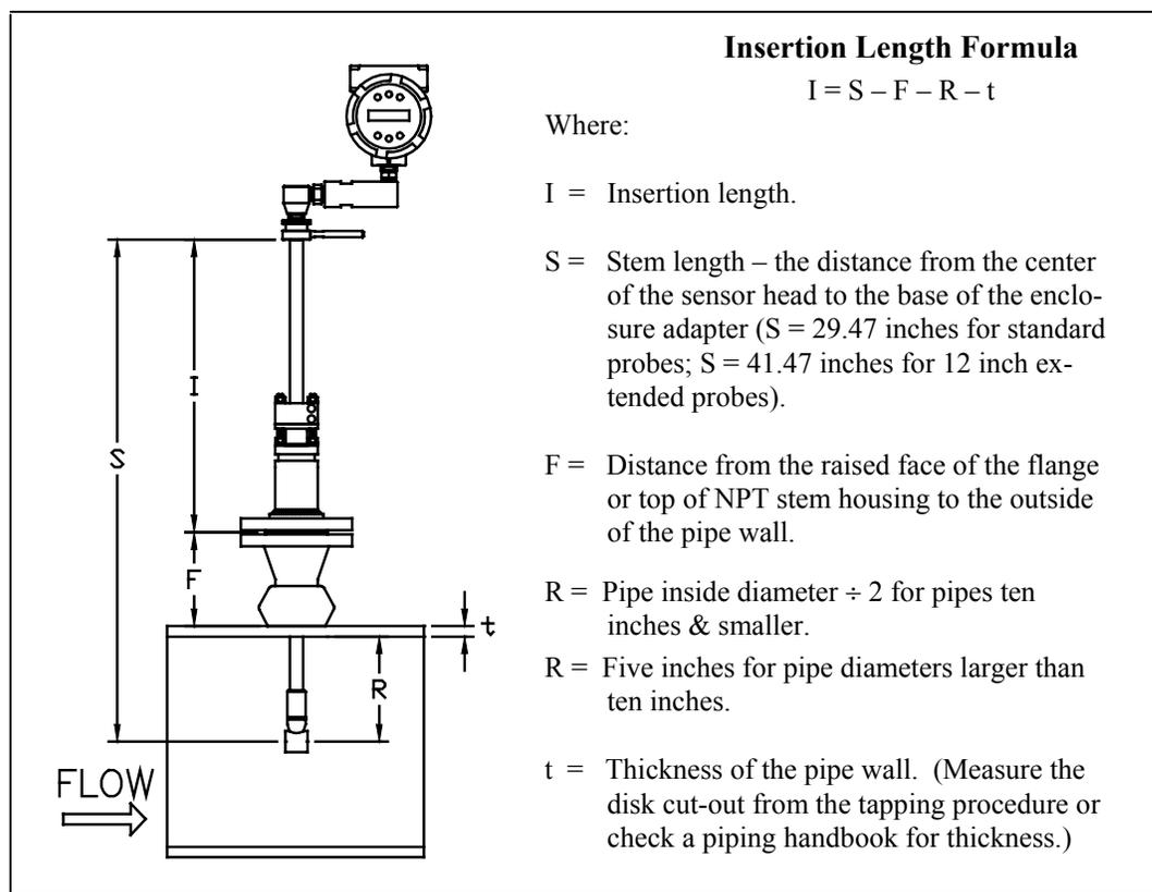
Figure 2-11. Insertion Calculation (Meters without Insertion Tool)
