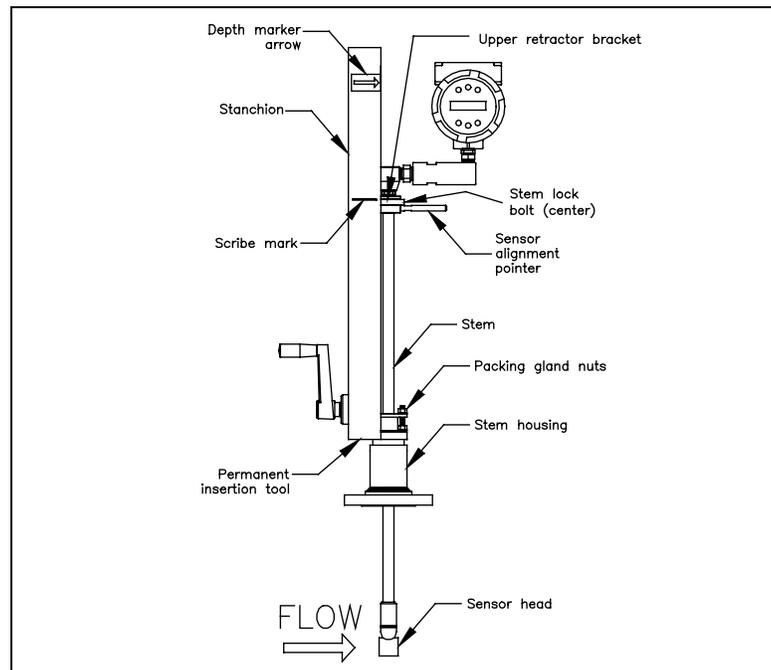
Figure 2-9. Flow Meter with Permanent Insertion Tool
