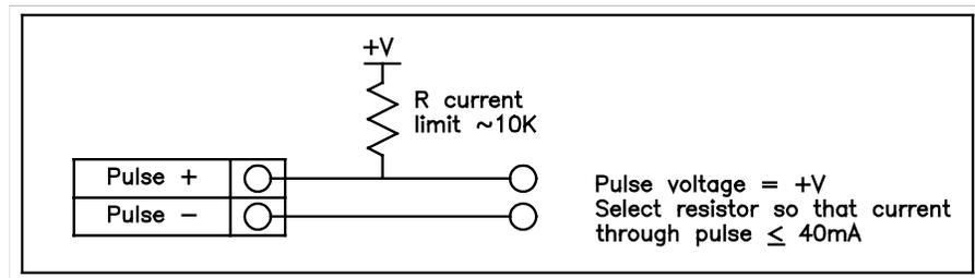
Figure 2-16. Isolated Pulse Output with External Power Supply
