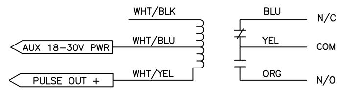
If you need a dry relay contact output you can drive a low powered 24 VDC relay (> 600  $\Omega$  coil) as above. The common Functional Devices Inc. RIBU1C relay shown above has been tested and works fine.
