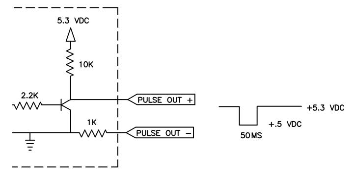
This drawing shows the pulse output circuit inside the Smart Electronics. Connecting directly to the 2 Pulse Output terminals provides enough drive to support a PLC digital input card or a simple self powered totalizer counter like a Red Lion CUB or a Omron H7EC series.
