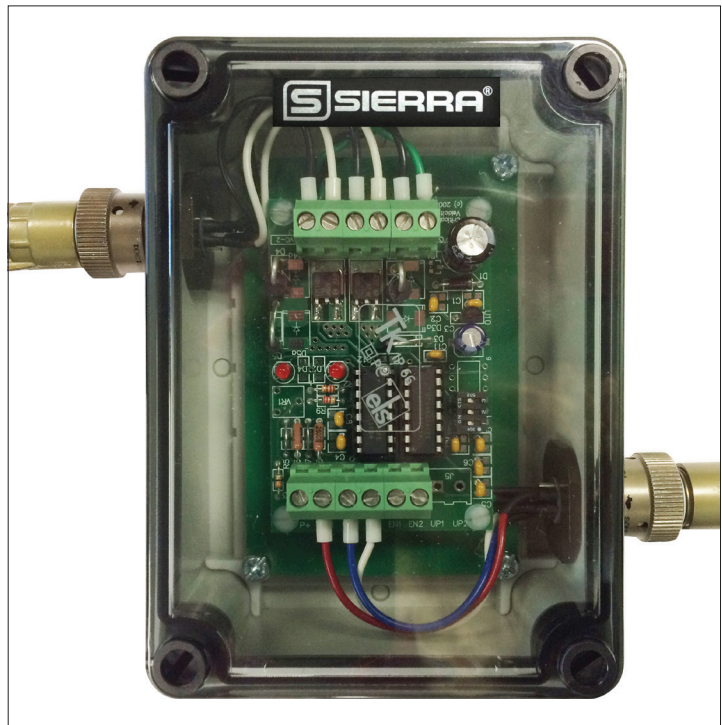
Figure 2a. NEMA 4X Enclosure for Control Circuit.
