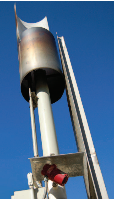
Sierra Steel-Mass™ 640S inserted into landfill flare
