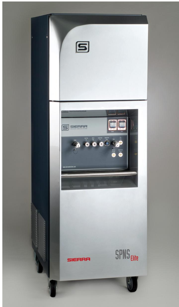
The SPNS was developed by SwRI in compliance with the United Nations Economic Commission for Europe (UN-ECE) regulations R49 and R83 for automotive emissions applications, and ICAO/SAE Air 6241 for aircraft emissions applications. SPNS technology has been used extensively by SwRI for over a decade in their own labs for engine emissions certifications and R&D purposes.
