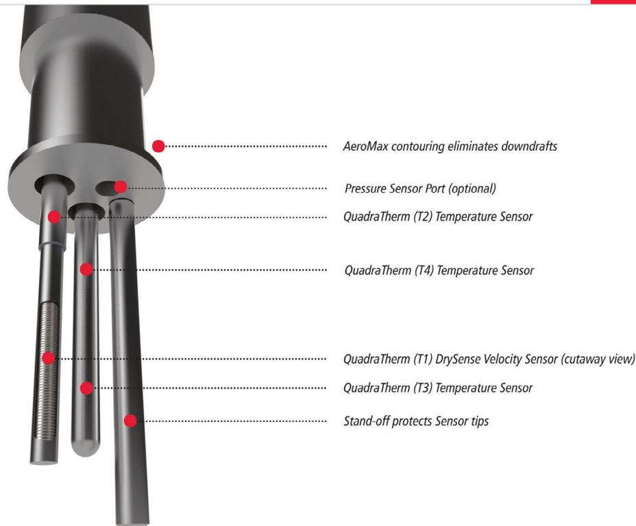
Figure 3. QuadraTherm® Four-Sensor Thermal Dispersion Sensor by Sierra Instruments
