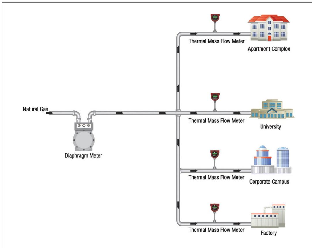
Figure 2. Sub-Metering Natural Gas to Mid-Size Facilities
